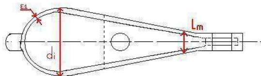
Diam.Di = 90 mm / Le, = ~500 mm / Lm, = ~ 40 mm / Pi = 80 mm
