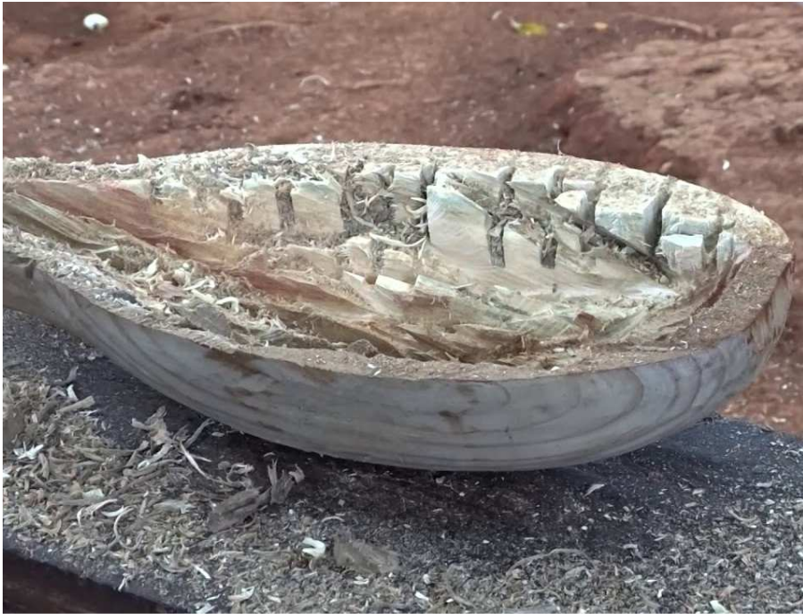
Maker Colo HASSANI (Chiconi, Mahore), while carving the soundbox with the chainsaw
