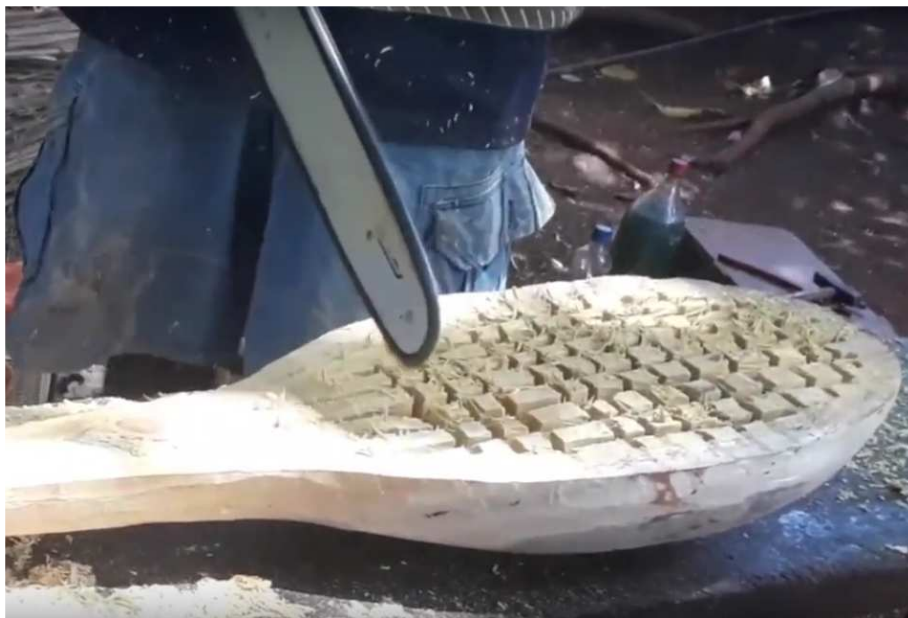
Maker Colo HASSANI (Chiconi, Mahore), while carving the soundbox with the chainsaw
