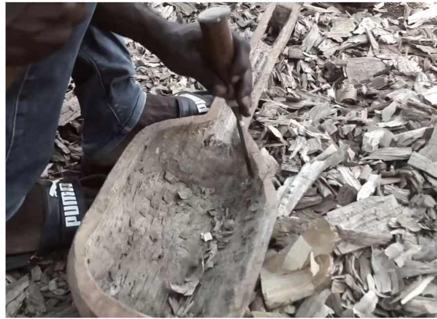
Maker BAYNA (Kaweni, Mahore), while finishing the soundbox with the gouge
