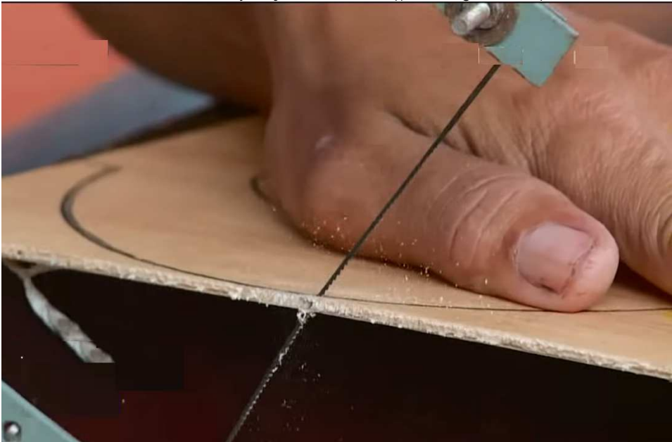
Cutting the resonator. Guitar Maker Fajar WIJAYA (Natar, Bandar Lampung), 2021
