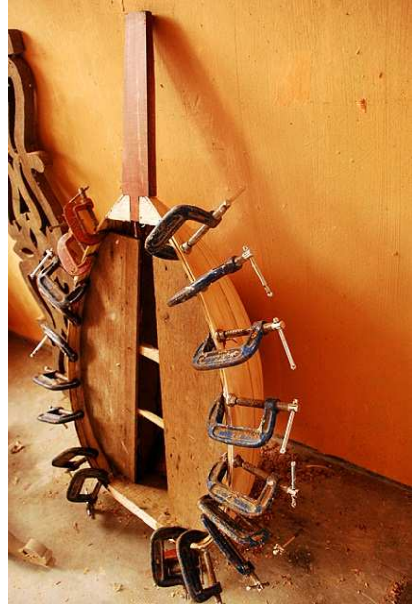
Clamps are holding outter ribs of a Gambus Hadramawt soundbox. Maker Mohamad Diah ARIFFIN, or "Pak Mat" in Kampung Rahmat, Batu Pahat, Johore state (picture by unknown web source)
