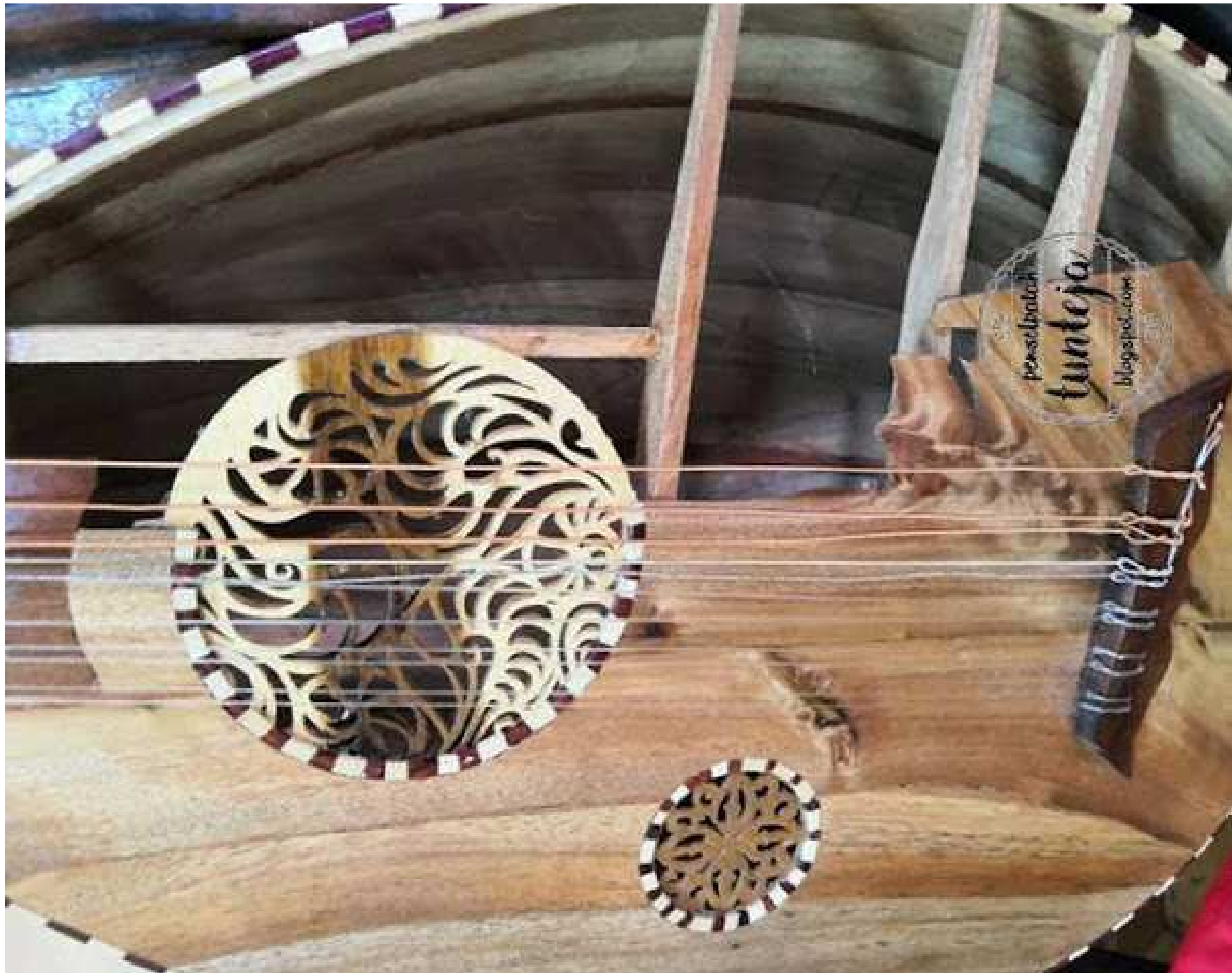
Exploded view, here showing the strengtheners of a Gambus soundboard (Maker HALIDAN, Johor)
