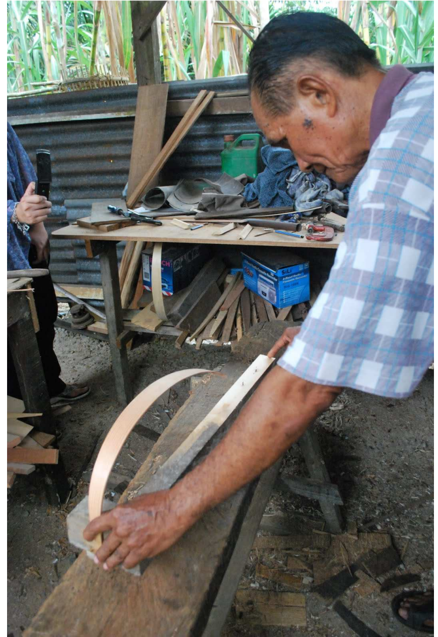
Assistant of “Pak Mat” ( Batu Pahat) while shaping the very first rib on the body (picture by web source)
