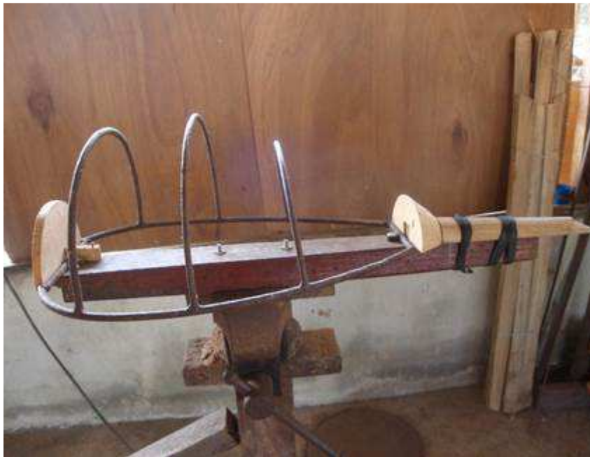
Photo 3.4.2 : final position of the shoulder, the neck and the bottom holder on the mould.
