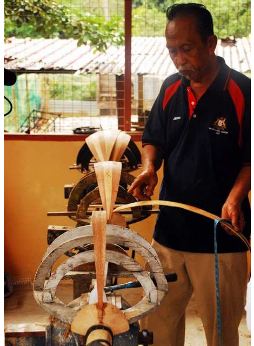
Conventional assembly of the soundbox of a arched back Gambus Hadhramawt lute. Maker Mohamad Diah ARIFFIN, or "Pak Mat" in Kg Rahmat, Batu Pahat, Johore. (picture by web source)
