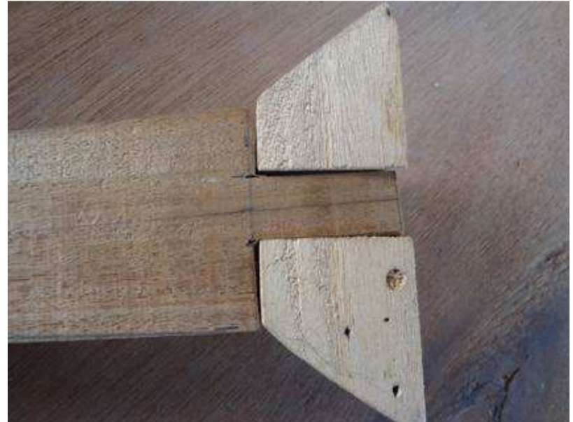
Photo 3.3.4: fitting the neck in the "shoulder"
