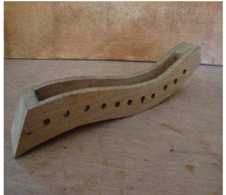
Photo 3.6.5 Holes for placing the ears harp
