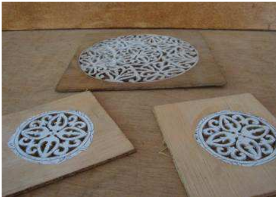
Photo 3.9.1: The paper patterns are pasted of the surface of the plywood prior cutting.
