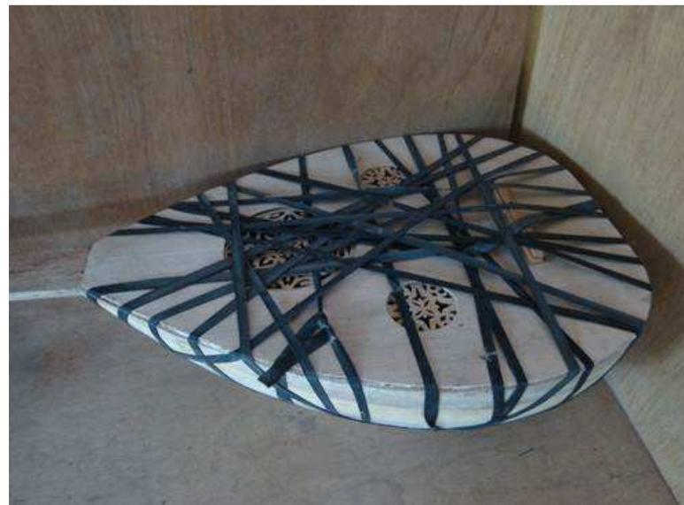
Photo 3.11.1: The soundboard is pressed on the sonbox with rubber straps
