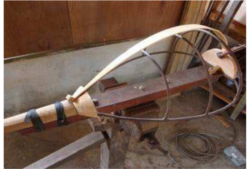
Photos 3.5.4 Strapping the blade on the mold with a rubber strap
