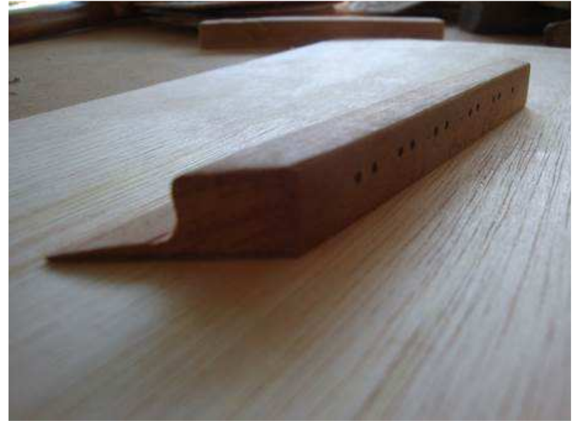
Photo 3.10.3: String holes have been drilled
