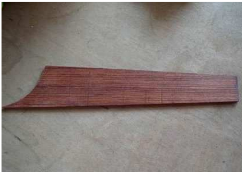
Photo 3.12.1: Covering the fingerboard with a rosewooden flat board
