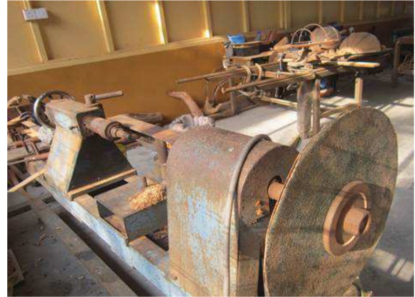
Photo 3.12.3: The engined turning device
