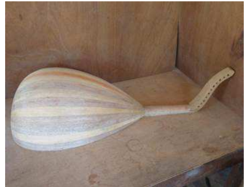
Photo 3.6.7: the lute after assembly of the pegbox
