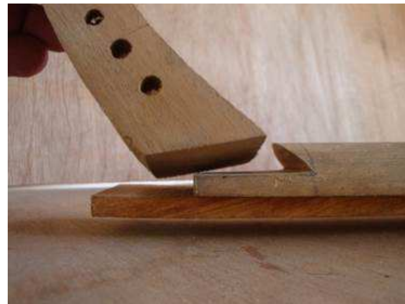
Photo 3.6.6 Final assembly of the pegbox.
