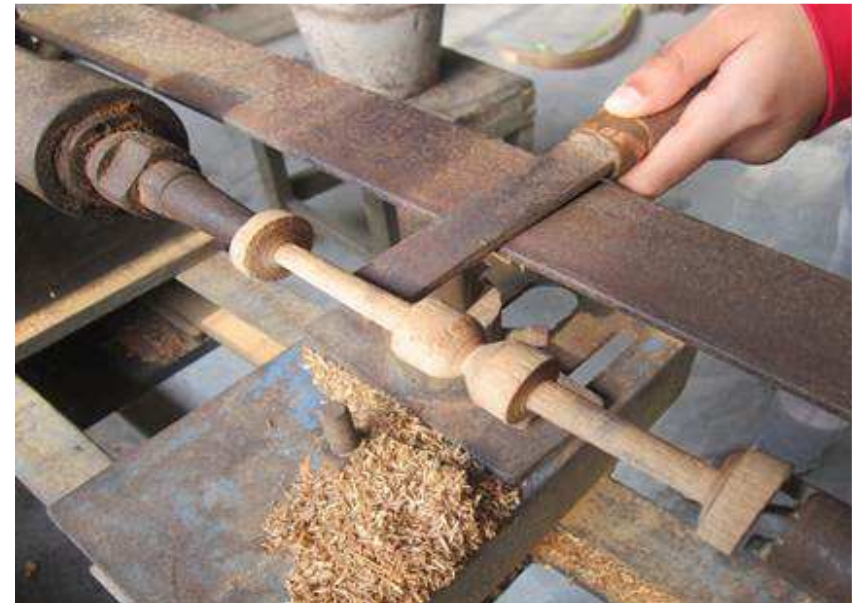
Photo 3.12.4: Turning the pegs
