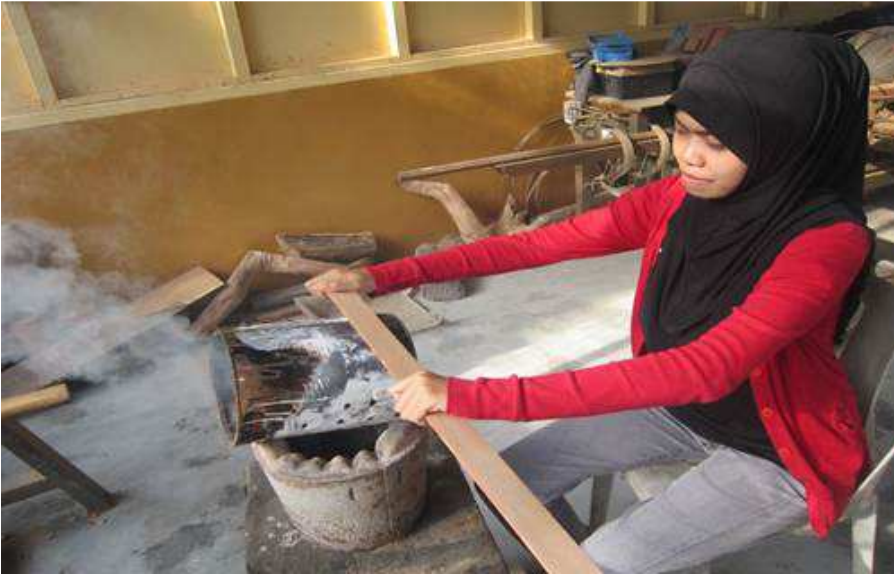
Photo 3.5.1 The maker while bending the wooden rib on the heater.
