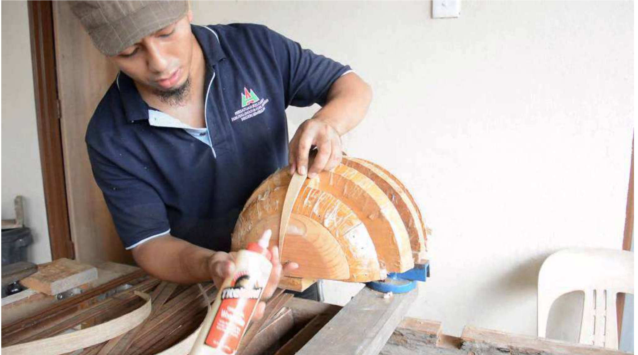
Adjusting the very first rib on a Gambus Hadramawt mold. Maker Mohamad Diah ARIFFIN, or "Pak Mat" in Kampung Rahmat, Batu Pahat, Johore state (picture by unknown web source)
