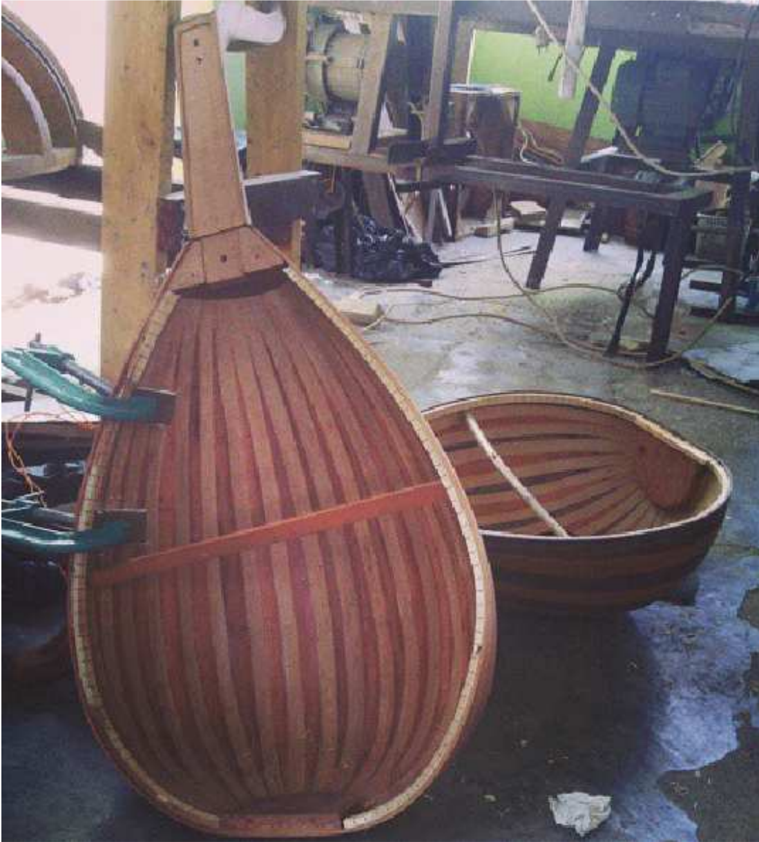
Clamps are holding outter ribs of a Gambus Hadramawt soundbox (picture by unknown web source)
