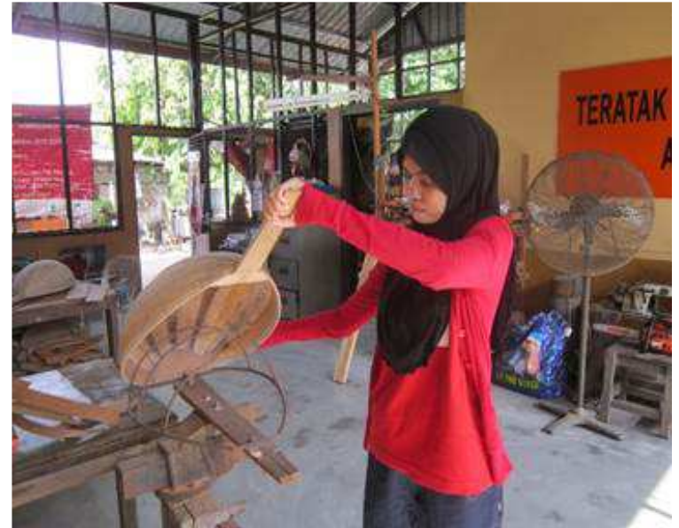
Photos 3.5.7 Lifting the body lute that is ready to unmold
