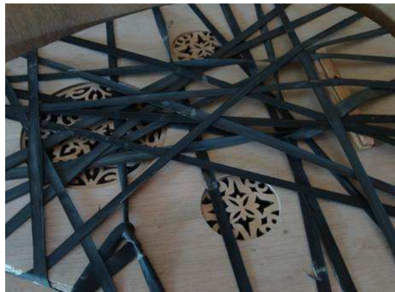
3.11.2: The soundboard is pressed on the sonbox with rubber straps
