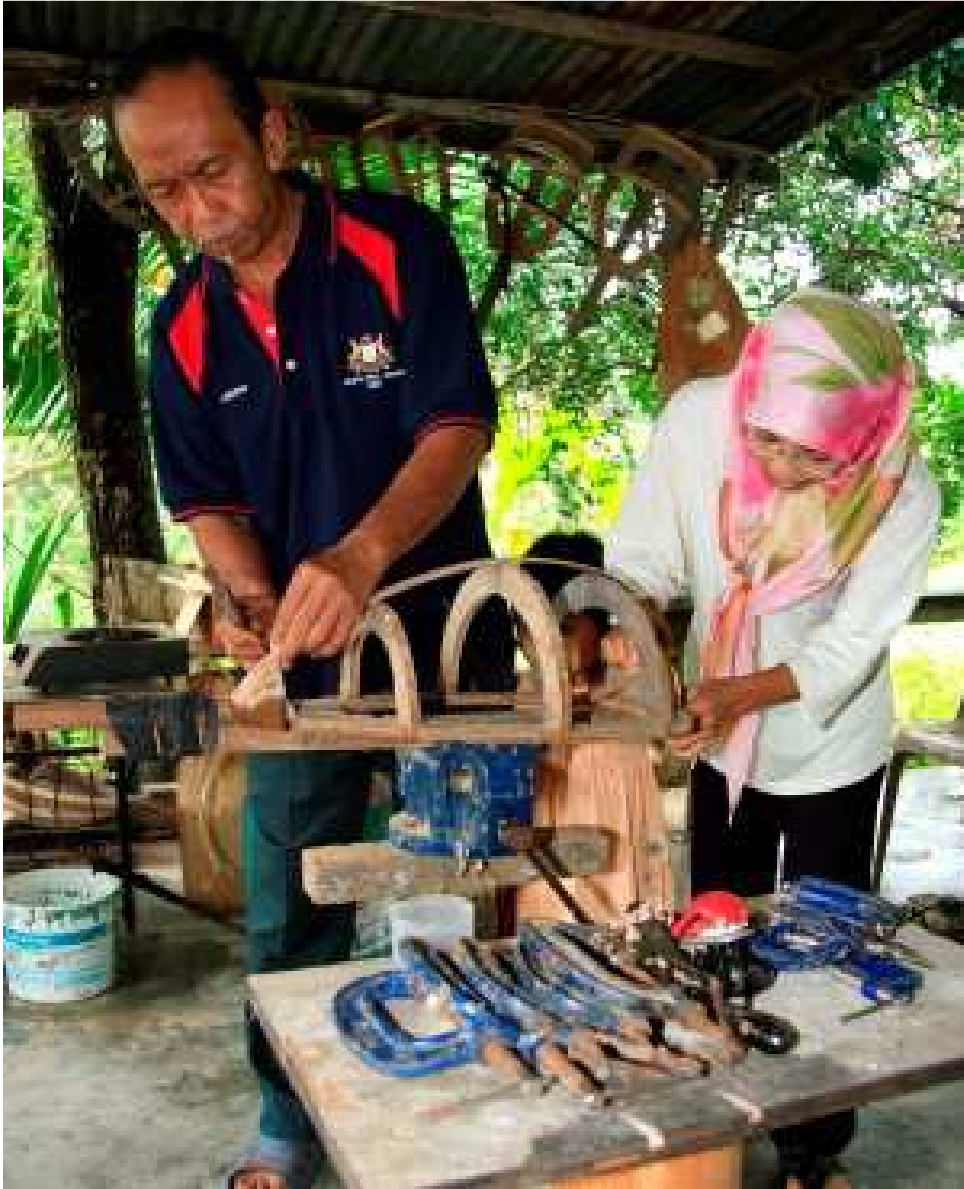
Lutemakers are fixing the first rib on the mould. Foreground : the related clamps. Maker Mohamad Diah ARIFFIN, or "Pak Mat" in Kampung Rahmat, Batu Pahat, Johore state. (picture by Krattfung Malaysia)
