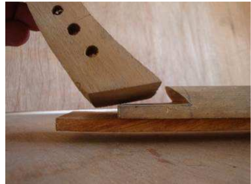
Photo 3.6.6 Final assembly of the pegbox.
