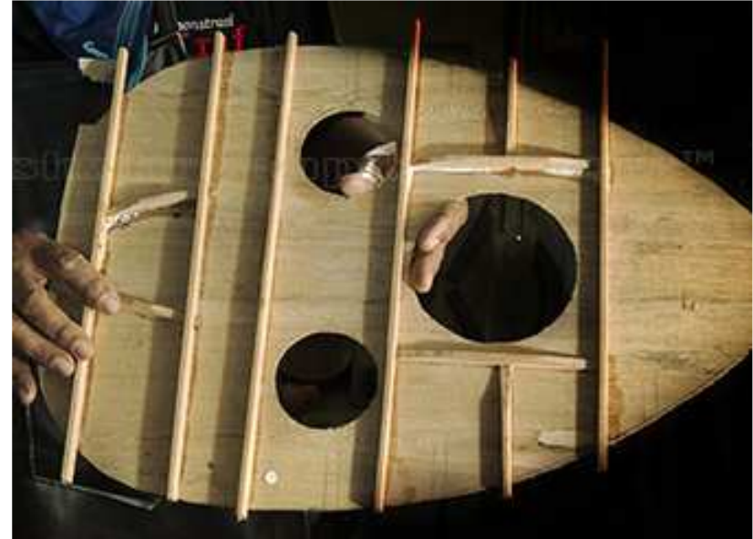
Strengtheners of a Gambus soundboard (Maker ARIFIN, Batu Pahat)
