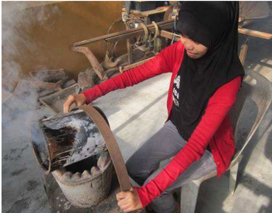
Photo 3.5.2 The hot blade becomes flexible under the effect of hot pipe.
