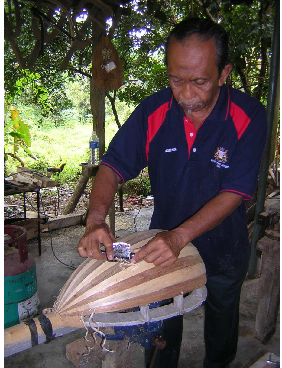
Polishing the soundbox. Maker Mohamad Diah ARIFFIN, or “Pak Mat” in Kampung Rahmat, Batu Pahat, Johore state (picture by unknown web source)
