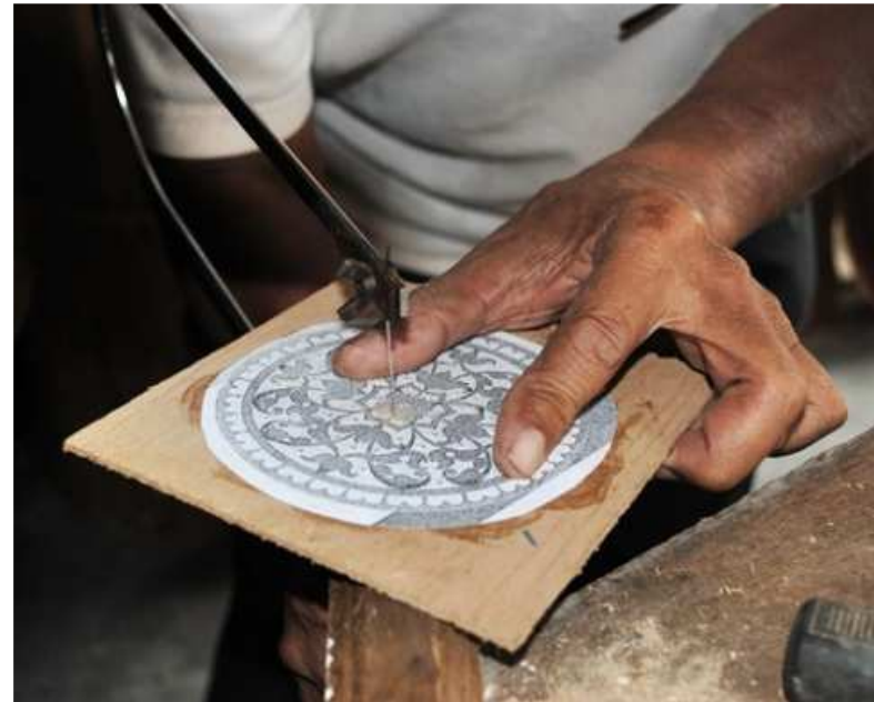
Shaping the rose out of a thin woodboard. Mohamad Diah ARIFFIN, Kampung Rahmat, Batu Pahat, Johore state. (picture by web source).
