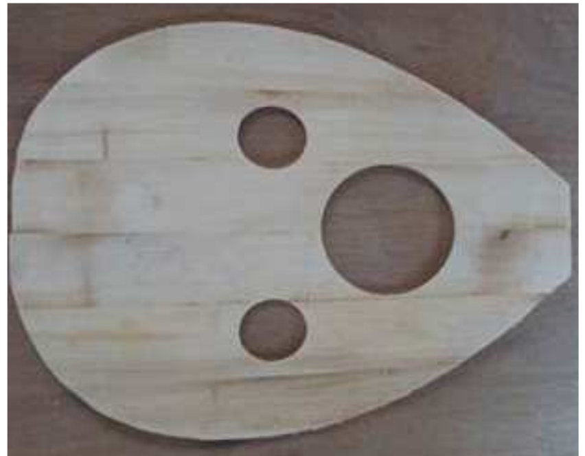
Photo 3.7.4 Cutting the soundholes
