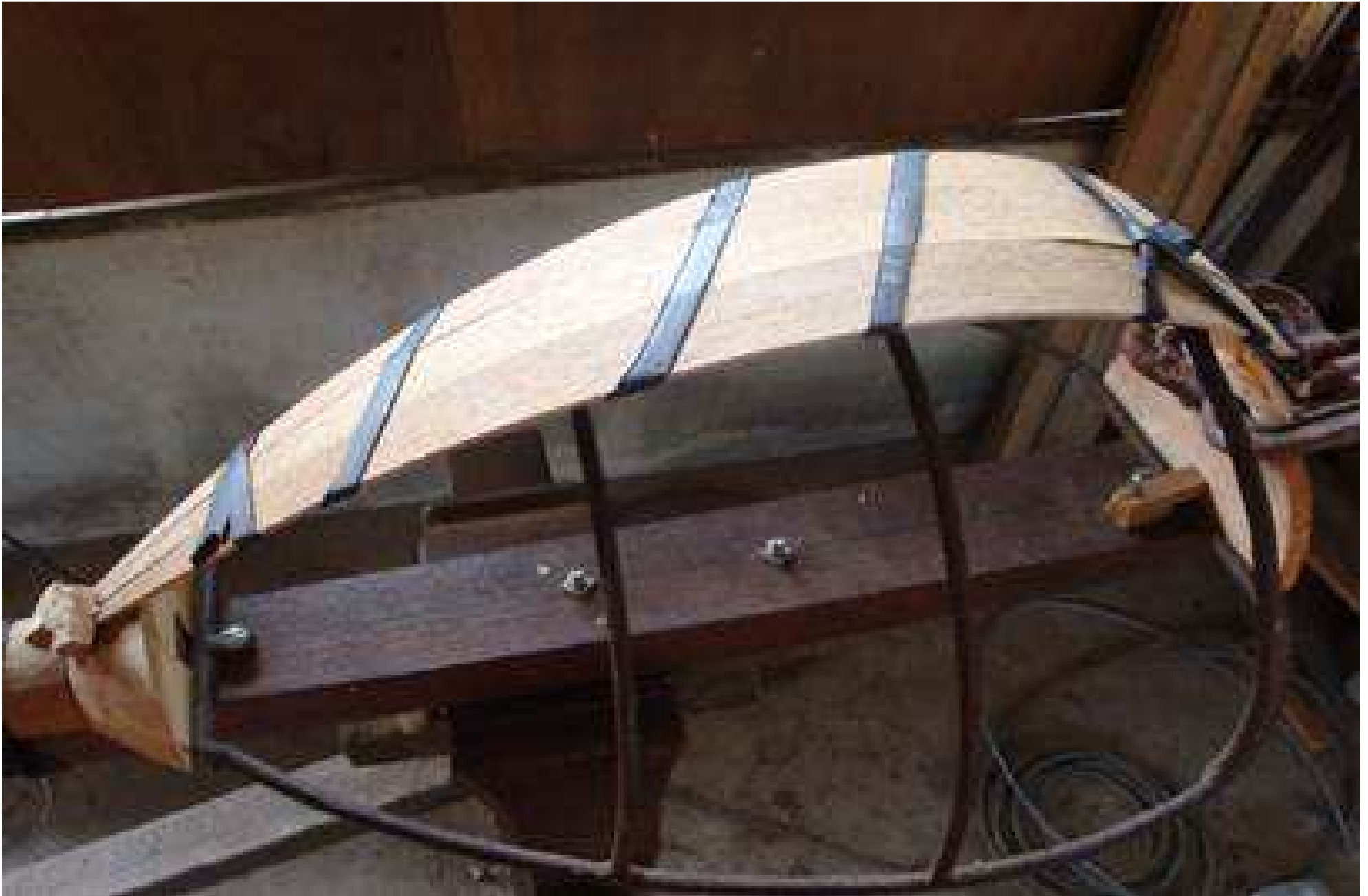
Photo 3.5.5: assembling the ribs on the mold. Note the numerous wooden clips.
