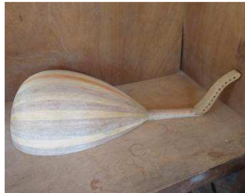
Photo 3.6.7: the lute after assembly of the pegbox
