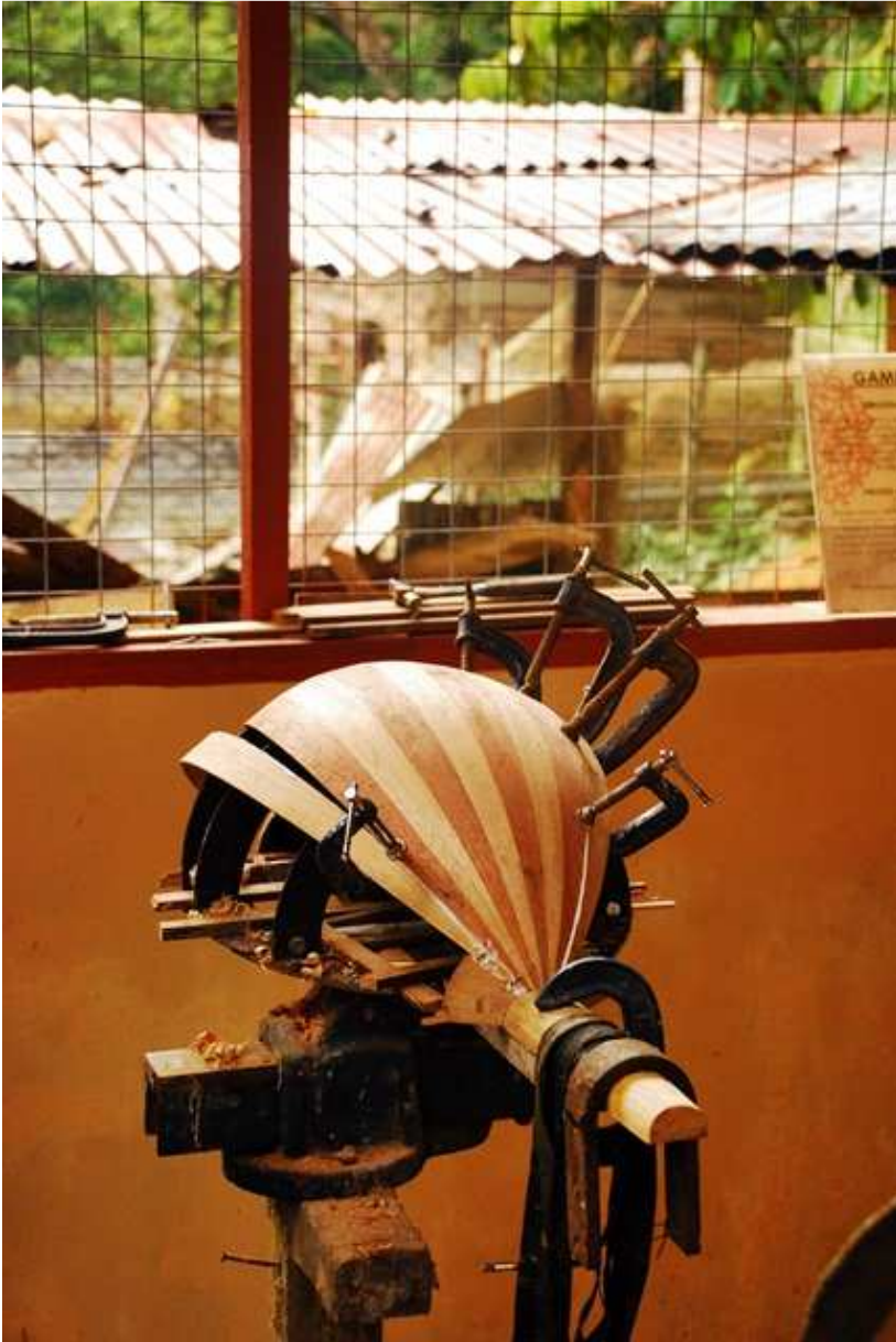
Clamps are holding outter ribs of a Gambus Hadramawt soundbox (picture by unknown web source)
