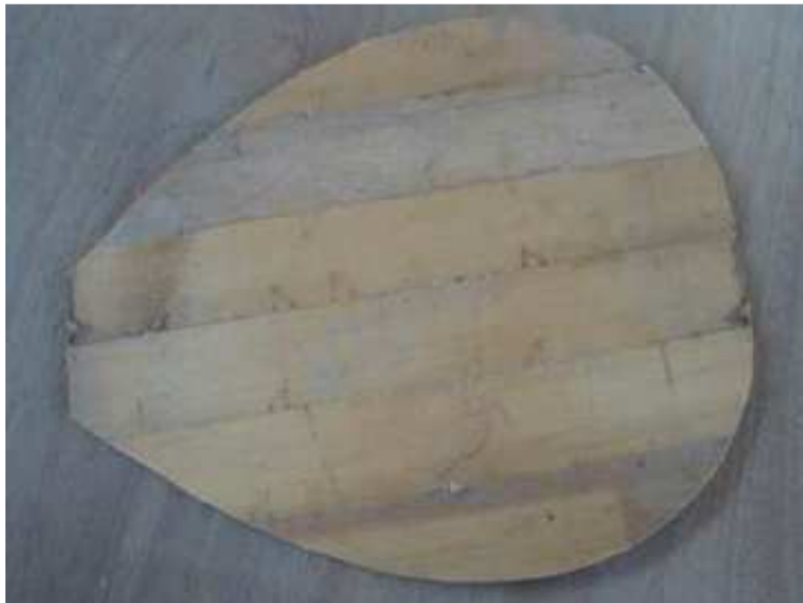
Photo 3.7.2 Board faces sketched by size and cut
