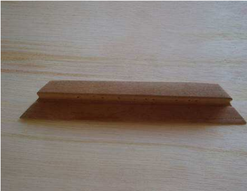
Photo 3.10.2: Shaping the tringholder out of an halban woodblock .
