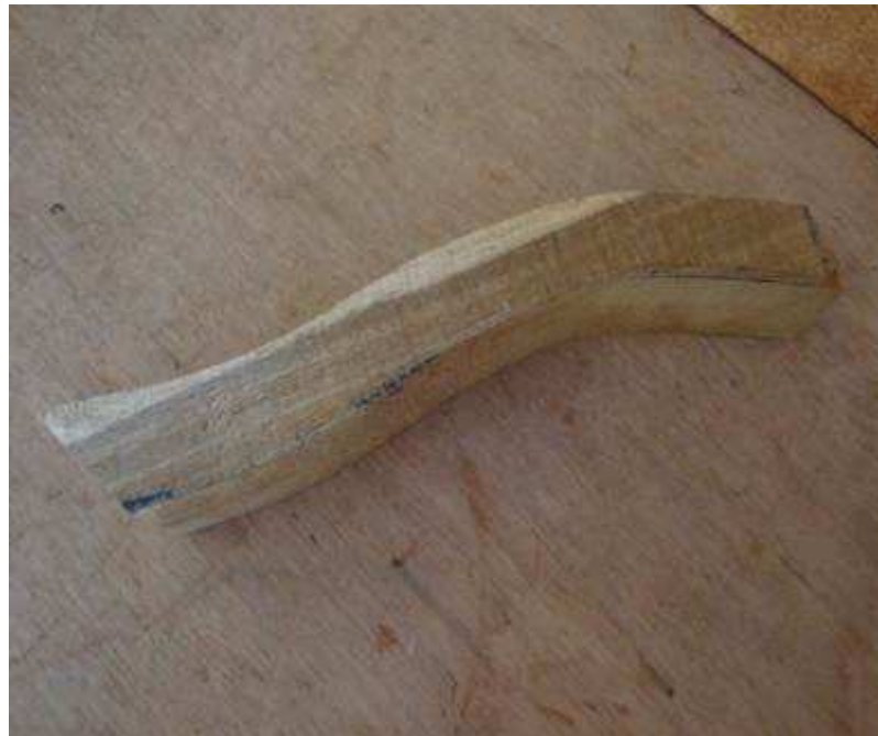
3.6.3 Side view after shaping the 'S' profile.
