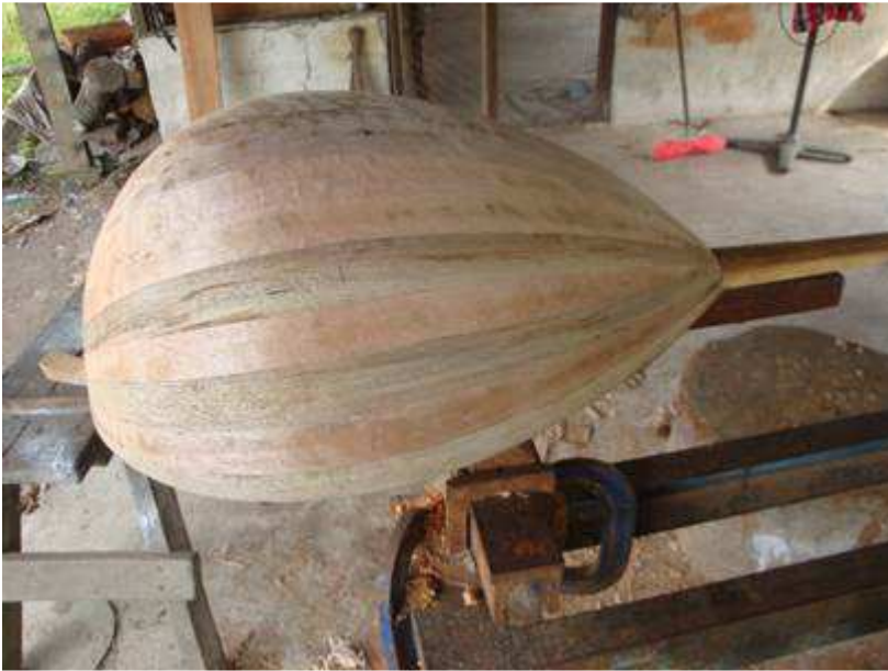
Photo 3.5.5: every blades are glued and assembled.
