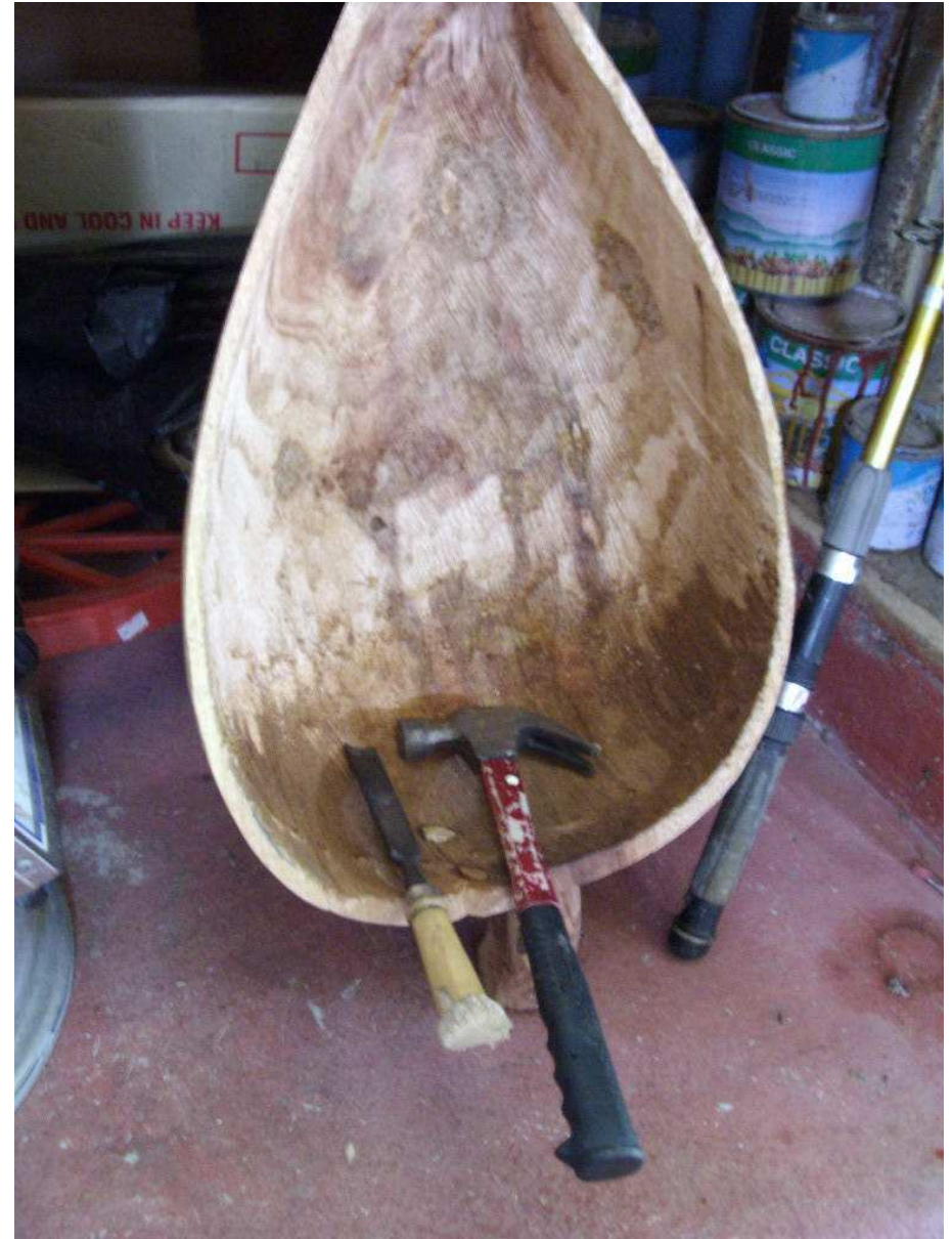
The box is handcarved with gouge. Average final thickness is about 8 -10 mm . Maker Awang PESAR, Seri Serbang, Bongawan, Sabah.
