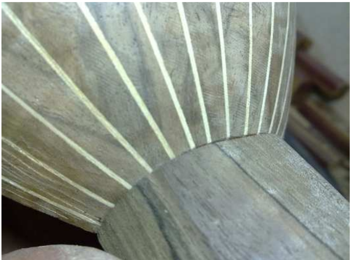
Maker is adjusting the gap between neck and body (Maker POURSHAGHAGHI, Iran)
