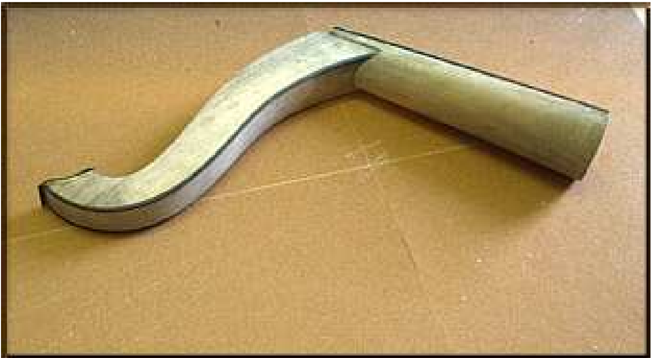
Assembling the Neck (glued dovetail). ( www.khalafoud.com )
