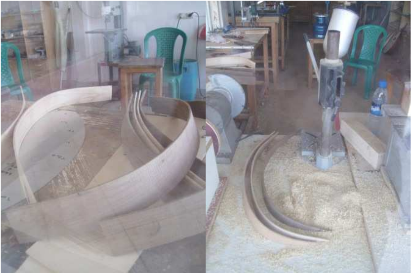
ASHARI used to cut the shaped ribs with an electrical cutter. Lutemaker ASHARI, bazar Ferdowsi, Bandar Qeshm, Hormuz Straits.
