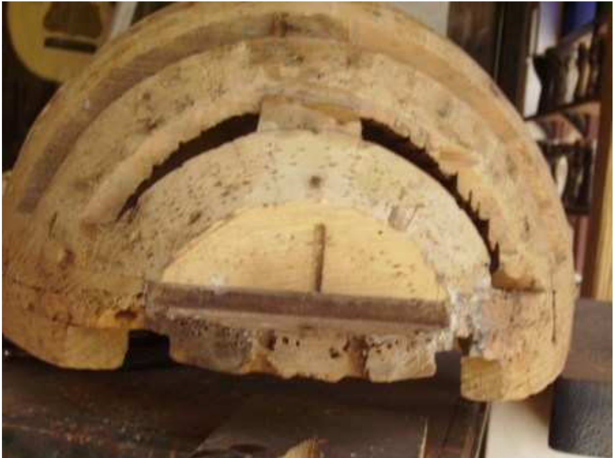
Soundboard pattern. The usual technic consists in assembling each rib with a clamp.
