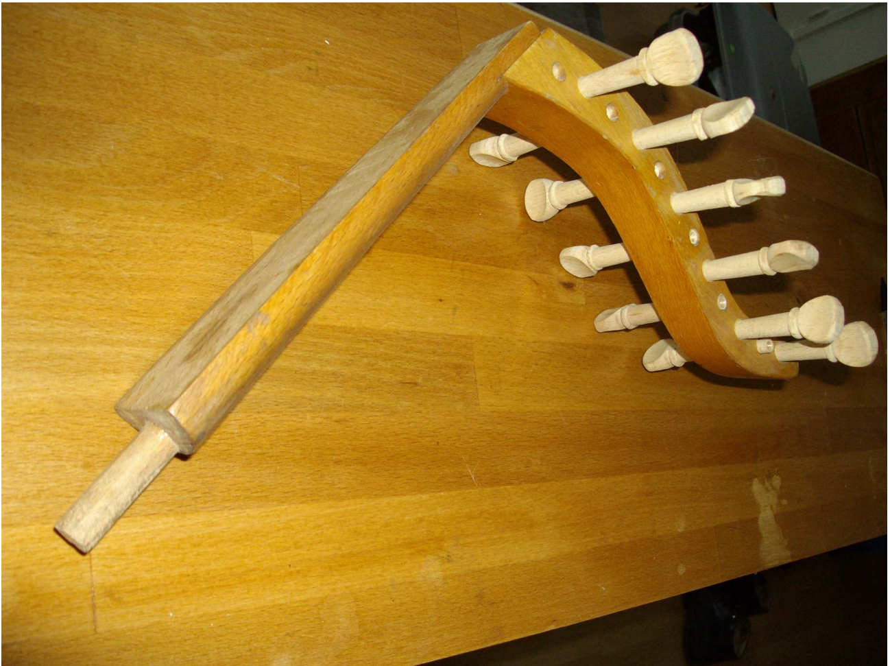
Assembling the Neck. Cylindrical variant of the dovetail from San'a, Yemen.
