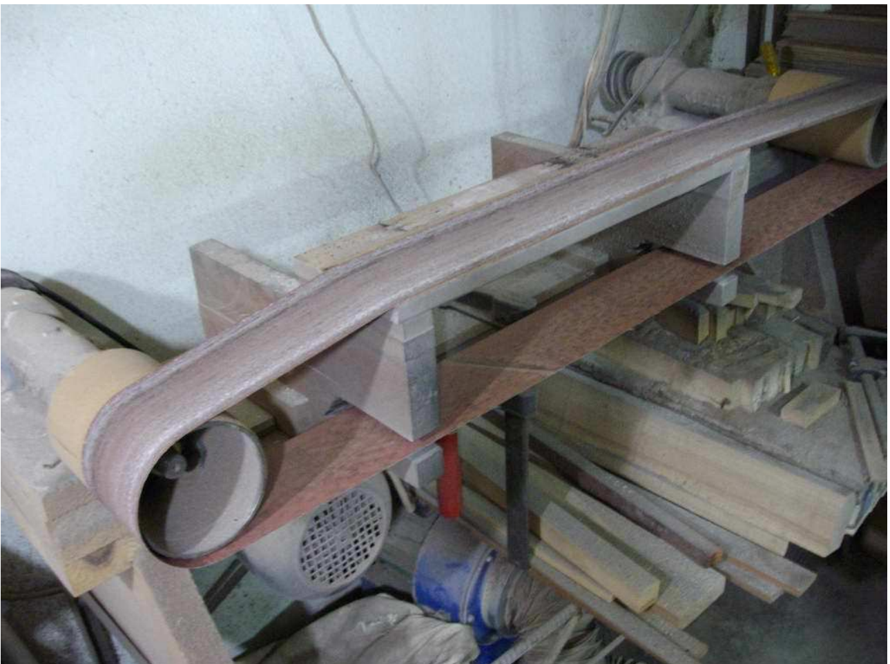
The soundboard is polished so that thickness doesn't exceed 2 mm. Dursun Ali NISADIR, Istanbul, Turkey.
