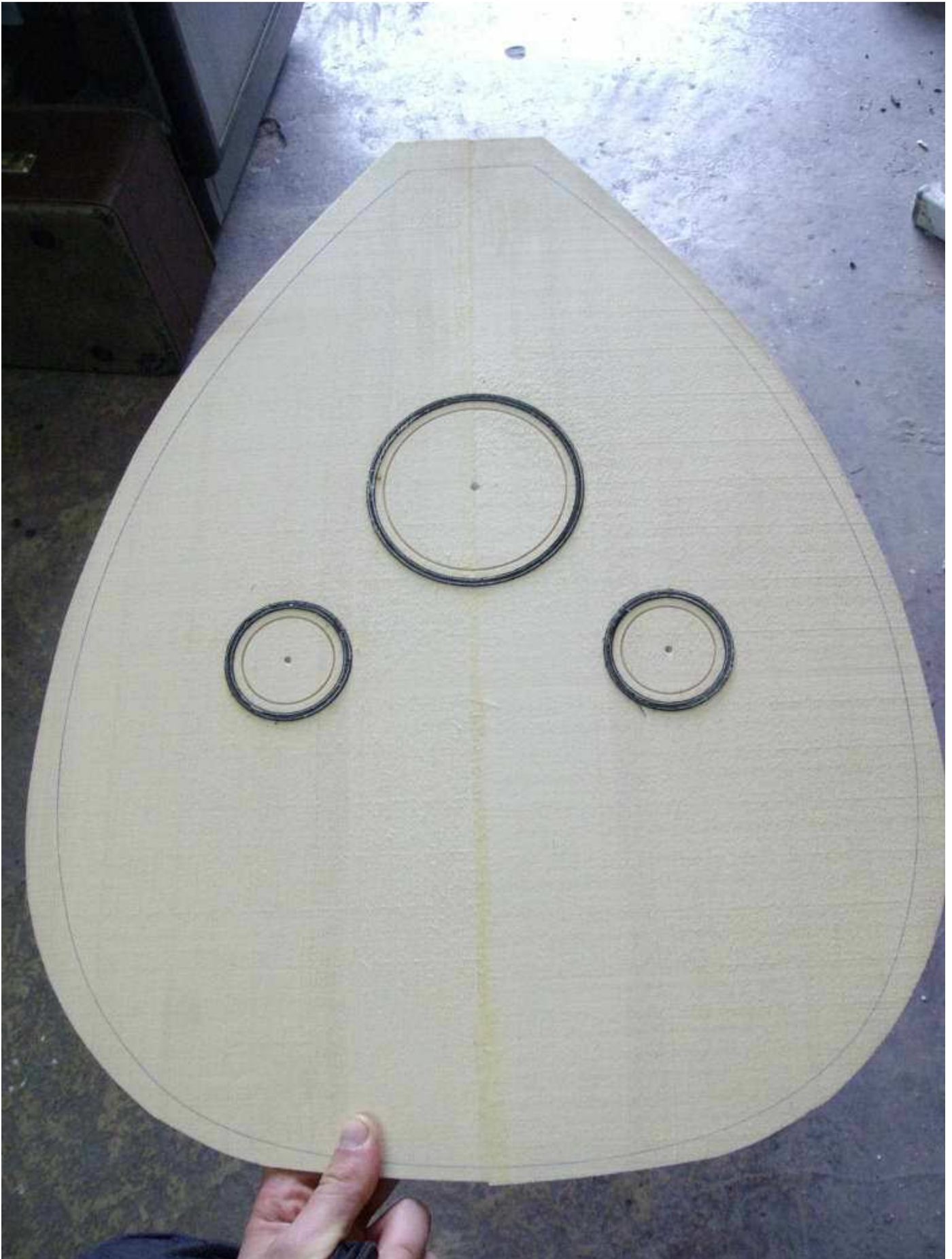
The soundboard is made of two glued ribs of pinewood. Maker Dursun Ali NISADIR, Istanbul, Turkey.
