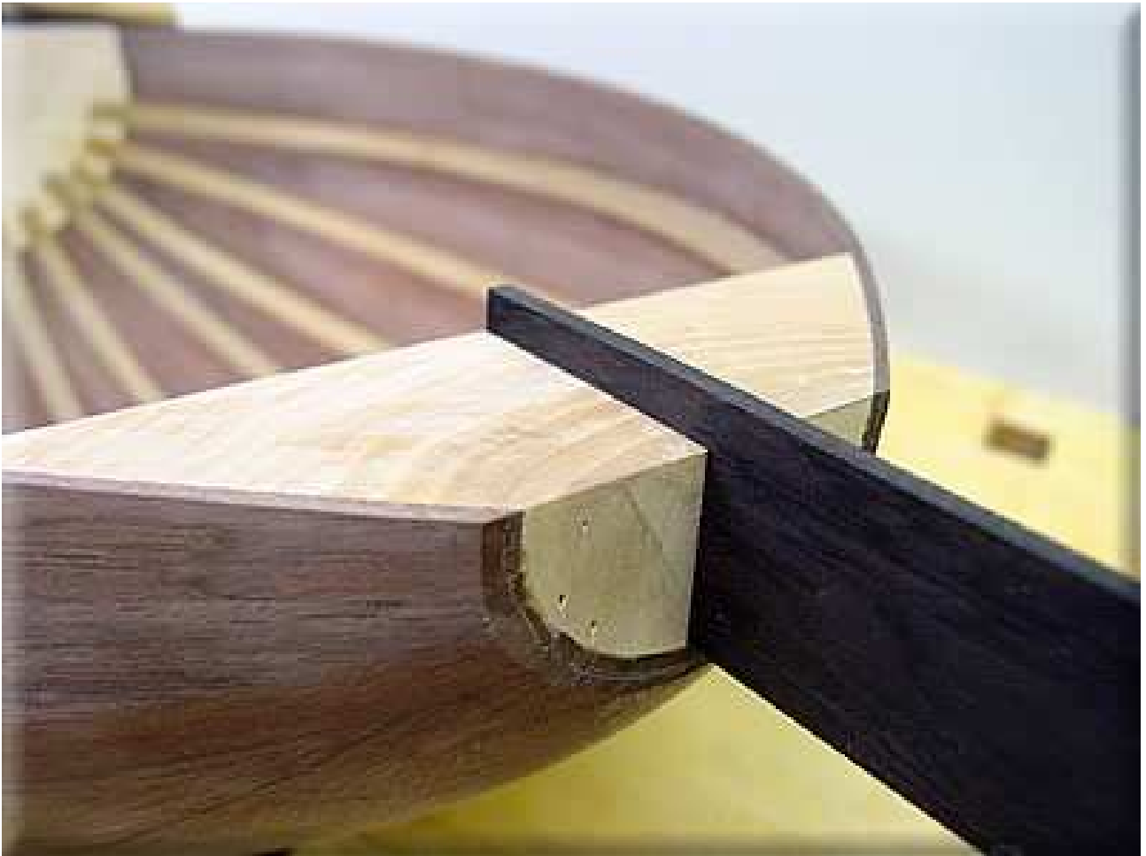
Assembling the Neck (glued dovetail). ( www.khalafoud.com )
