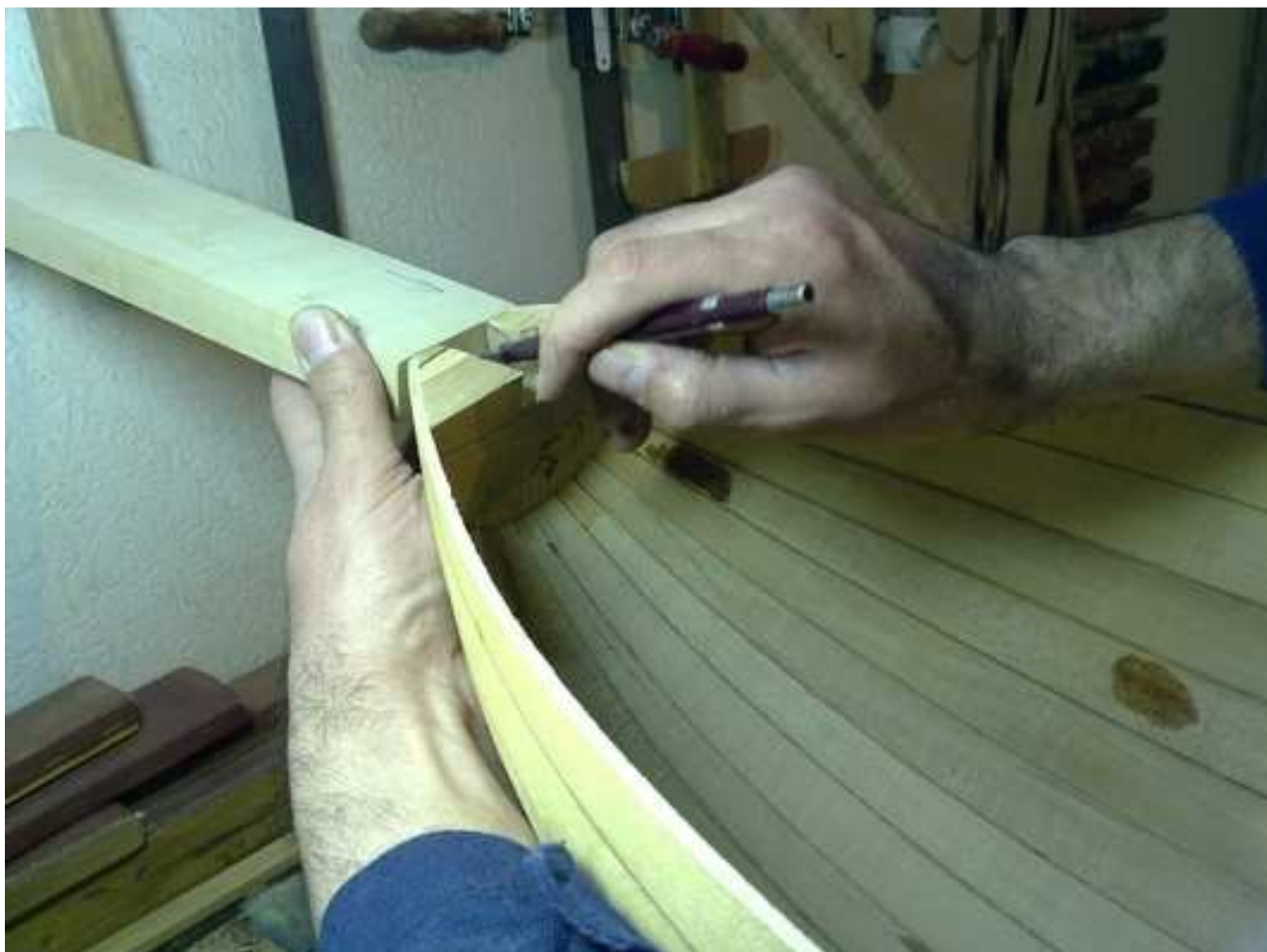
Shaping the Neck dovetail according the geometry of the soundbox. Maker POUSHAGHAGHI, Iran.
