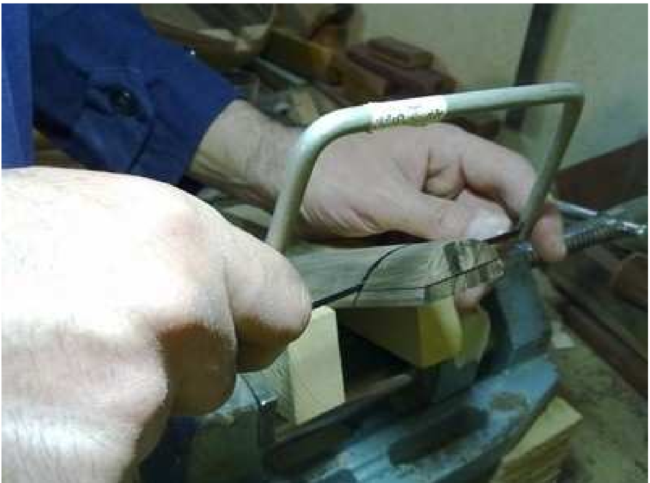
Cutting the Neck Head. Flat variant of the dovetail from Iran (maker POURSHAGHAGHI, Iran).
