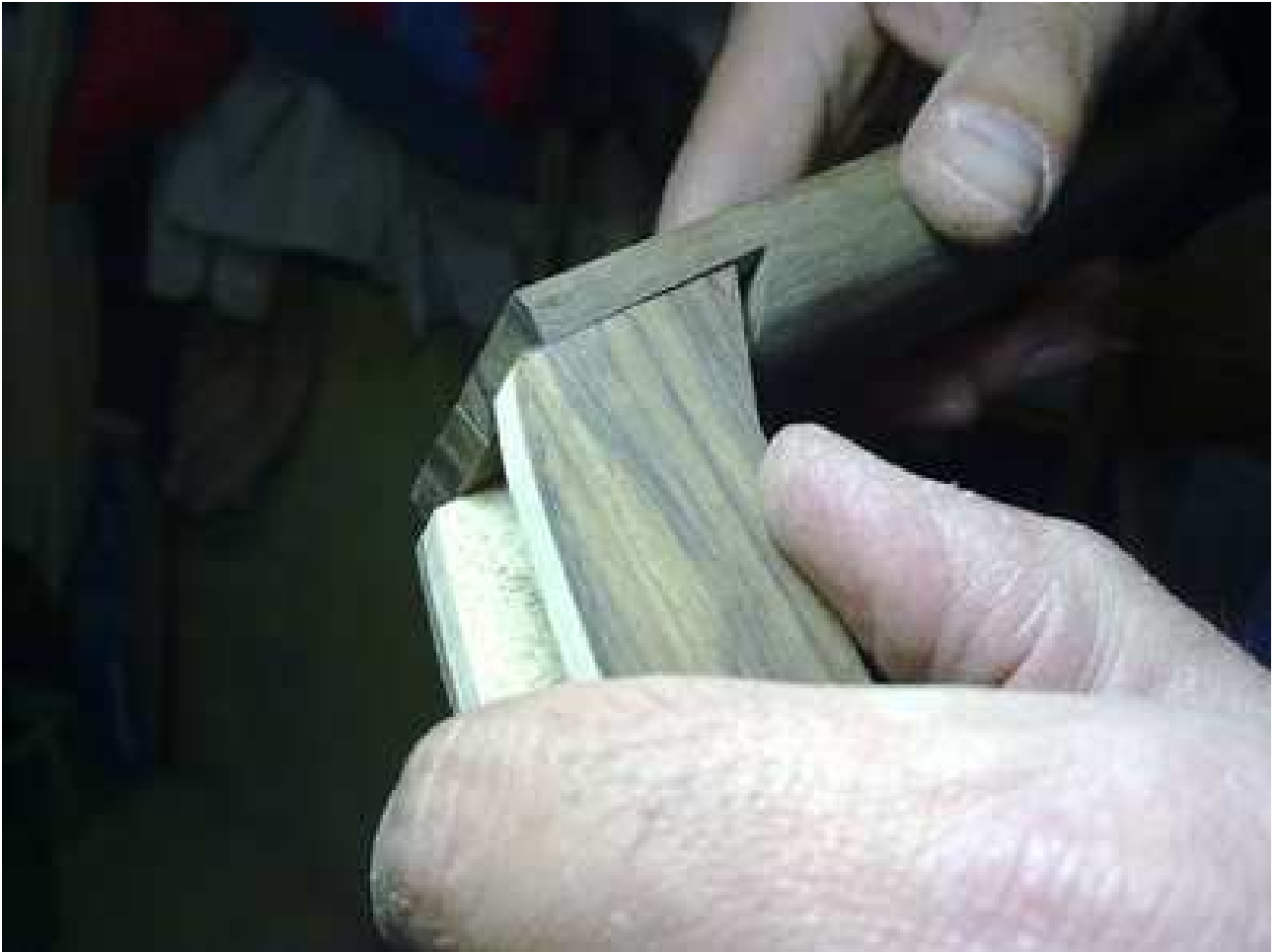
Assembling the pegbox on Neck. Flat variant of the dovetail from Iran (maker POURSHAGHAGHI, Iran).
