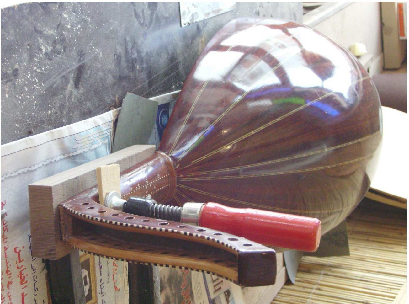
Assembling the Neck with clamp. Lutemaker in Doha, Qatar.
