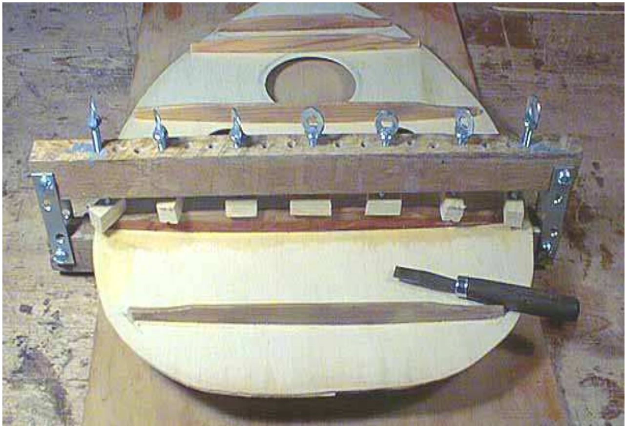
Clamps are needed , so that the inner ribs to be glued tightly. ( www.khalafoud.com )
