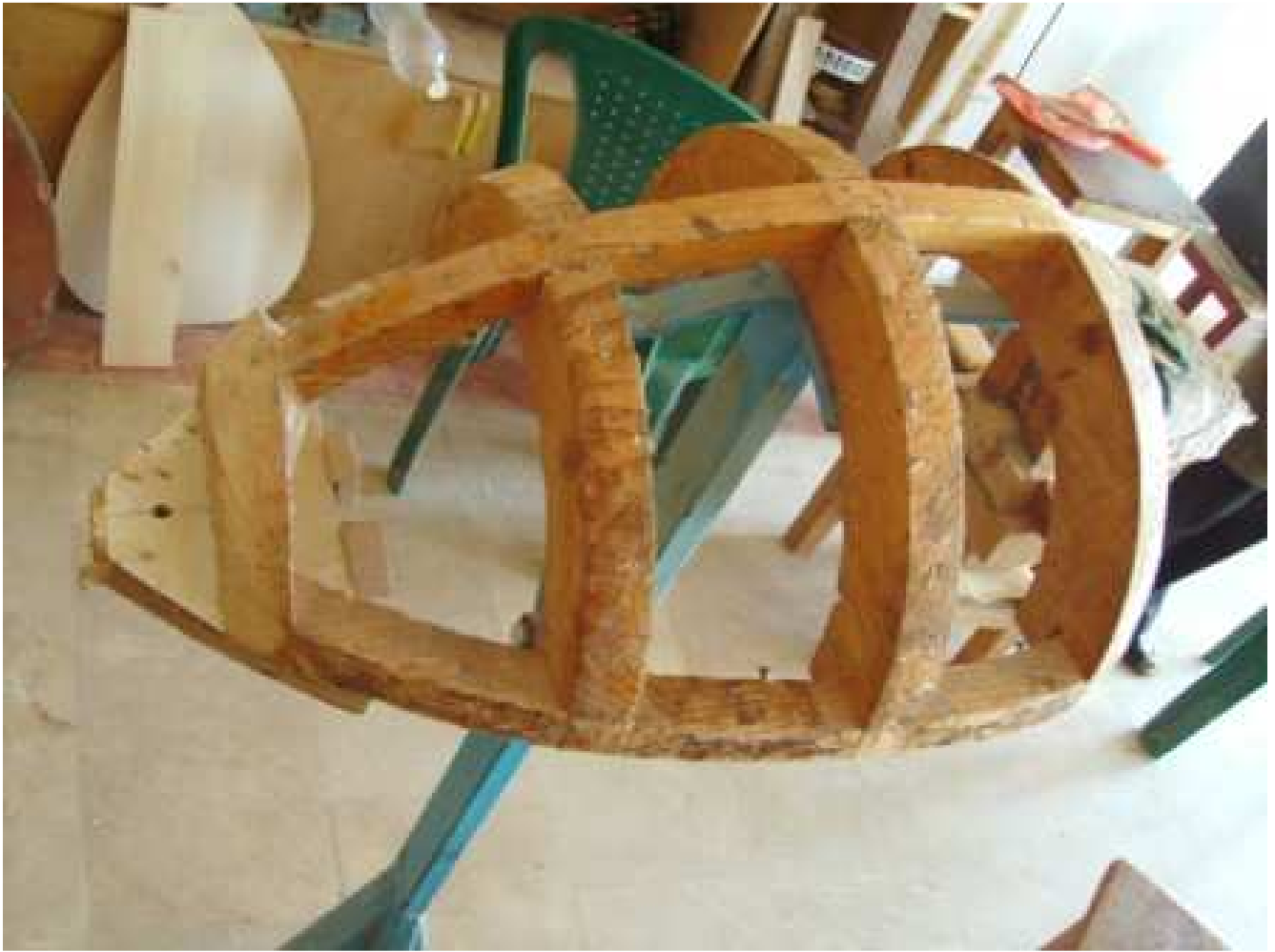
Oud soundbox pattern. Thanks to his efficient shaper / heater, Lutemaker "ASHARI" doesn't use any clamp.
