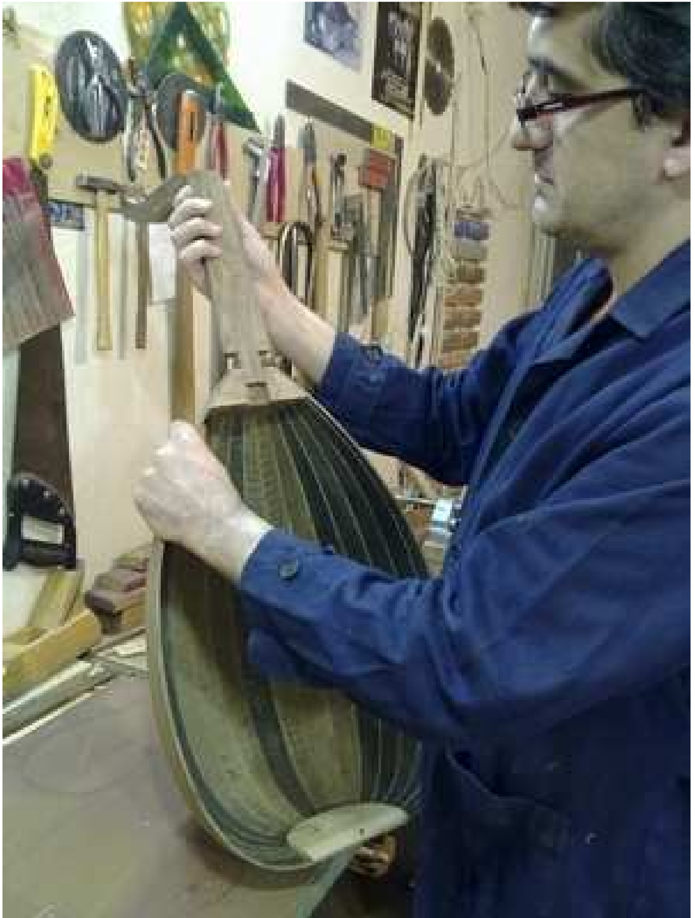
Adjusting the Neck on the soundbox. Maker POUSHAGHAGHI, Iran.
