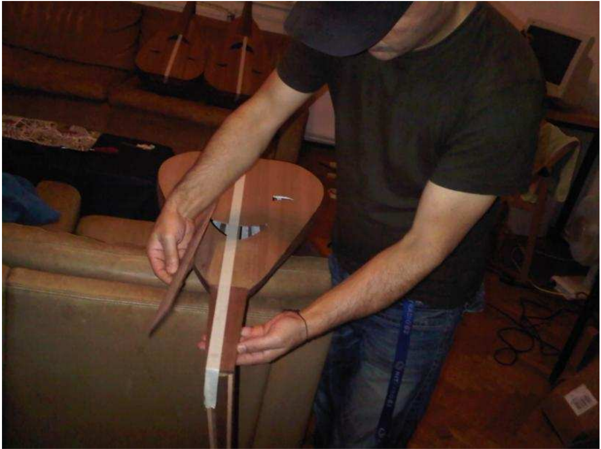
Adjusting a rose wood made fingerboard on the neck (Maker Mofid Nehmeh, Lebanon).
