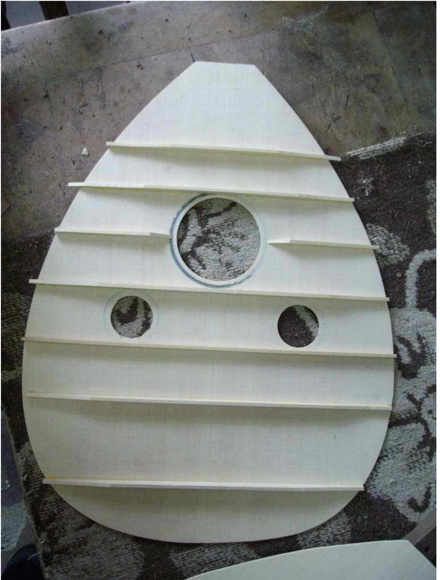
Strengthening the soundboard with pinewood bars, according to Dursun Ali NISADIR, Istanbul, Turkey. Former advices by ASHARI in the holder area are not applied here.
