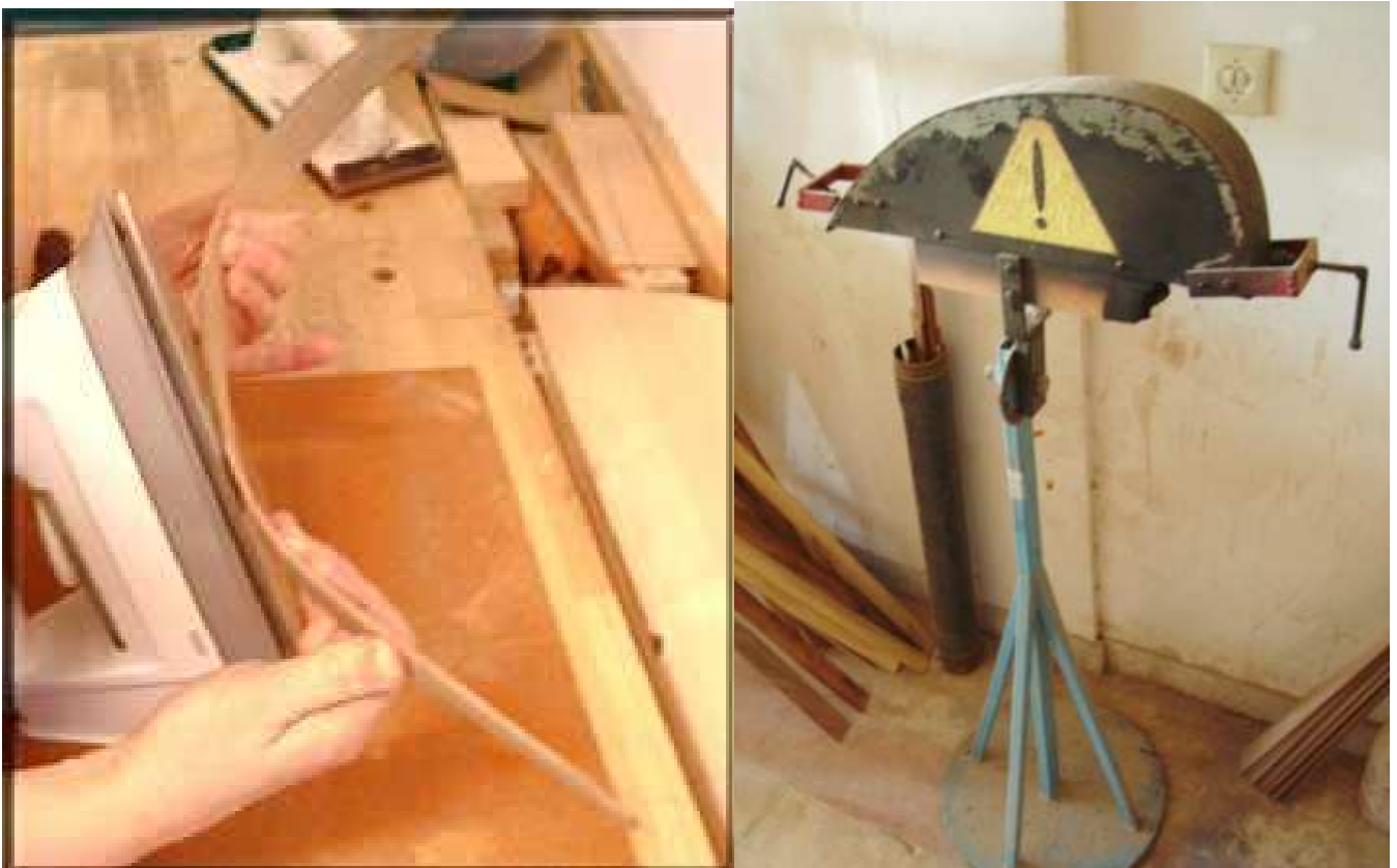
Left: An alternate technic is observed in Europe. Ribs are ironed after bath, then bended on the pattern by clamps or nails. Right : ASHARI manufactured this shape pattern / heater. Each wet rib is shaped after 45 minutes. Lutemaker ASHARI, bazar Ferdowsi, Bandar Qeshm, Hormuz Straits.
