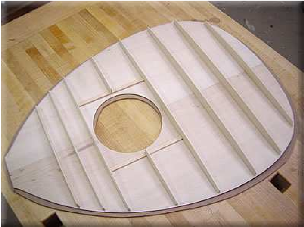
Glued ribs are spaced and strengthen the soundboard. . ( www.khalafoud.com )
