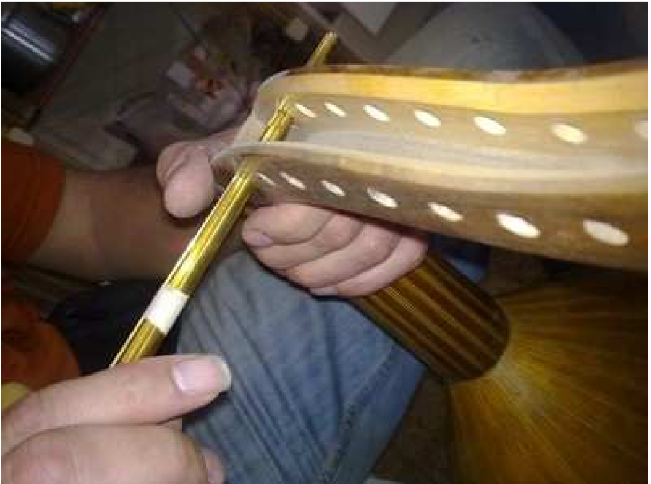
Adjusting the peg holes with a conical gauge (maker POURSHAGHAGHI, Iran).
