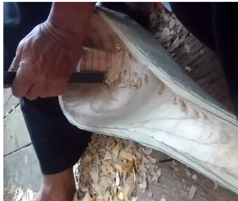
Hollowing out the soundbox (gouge), by maker SOOFIAN / “Busu PYAN” (JEMBAYAN)
