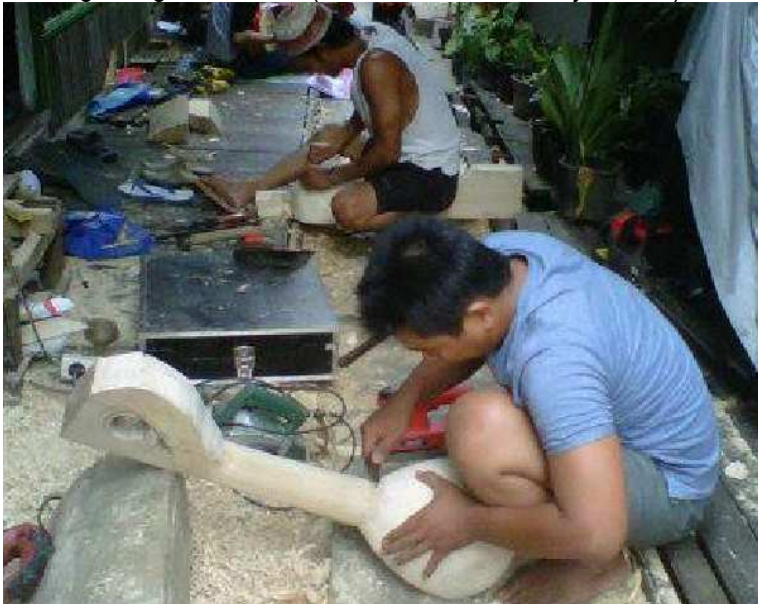
Carving out the body of a Panting . (maker Hidayat, Banjarmasin)
