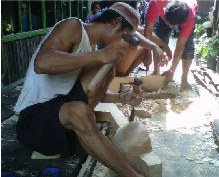
Carving a large soundbox (maker Hidayat, Banjarmasin)
