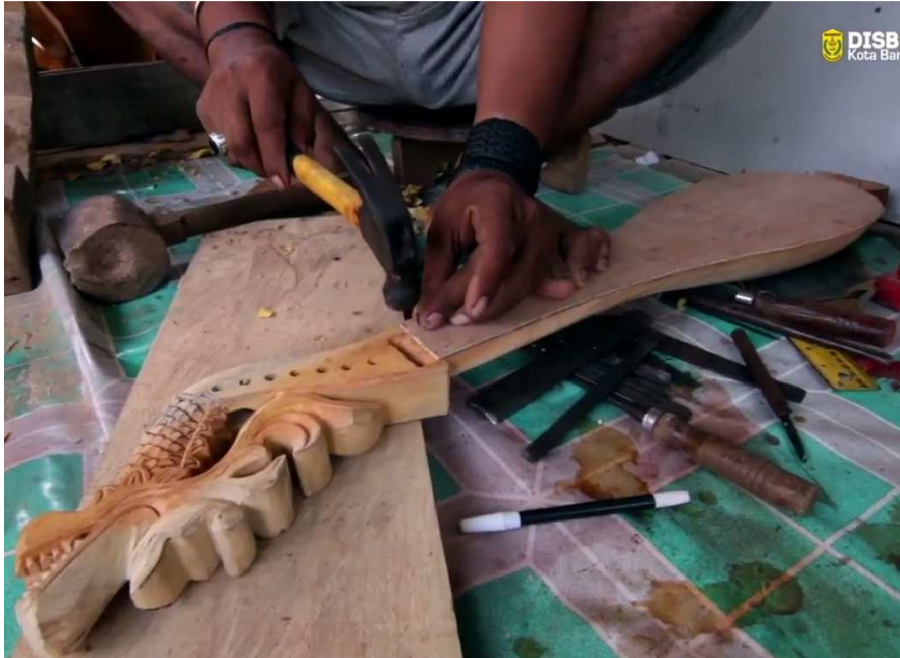
After shaping the wooden resonator, this is finally assembled. (maker HUSNI, Kota Banjarmasin)
