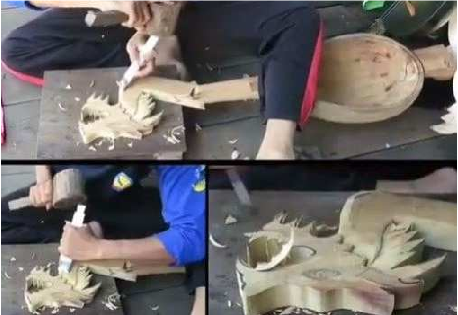
Carving the Naga head shaped pegbox (maker Fahrul ANWAR)
