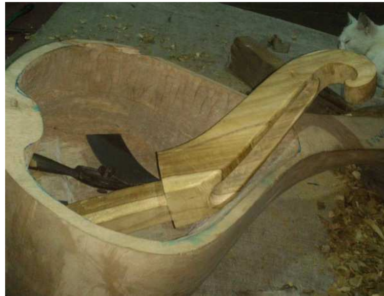
Panting pegbox assy (maker RUDDY a.k.a. "RURUD", Barikin)
