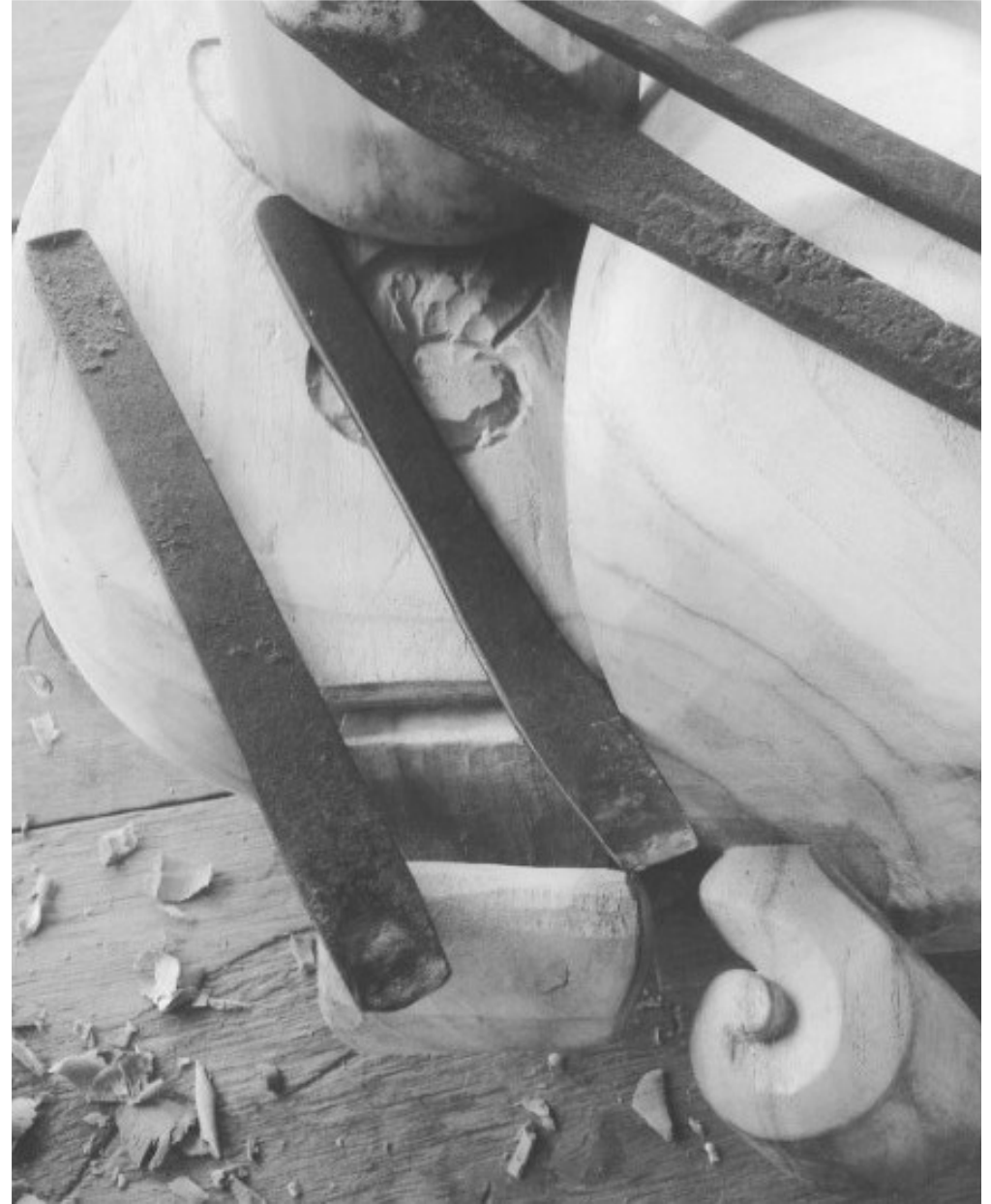
Shaping the stringholder (maker RUDDY a.k.a. “RURUD”, Barikin))
