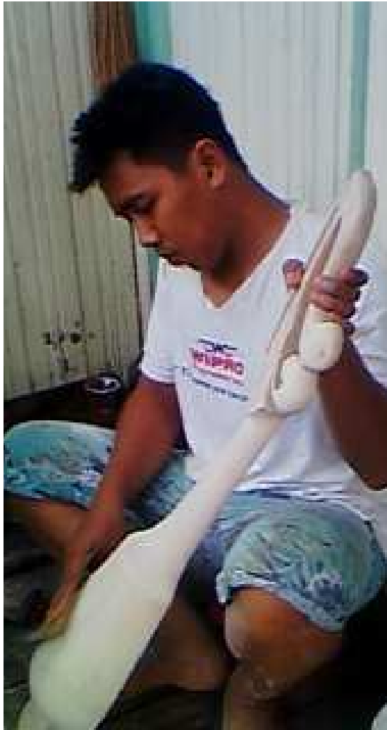
Varnisnig panting lutes (maker Masdar Hidayat in Banjarmasin, South Kalimantan)
