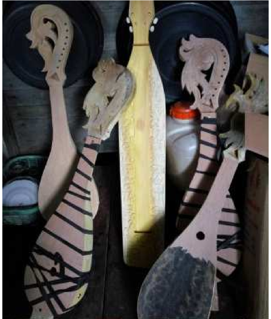
Glueing the fingerboard (maker Fahrul ANWAR)
