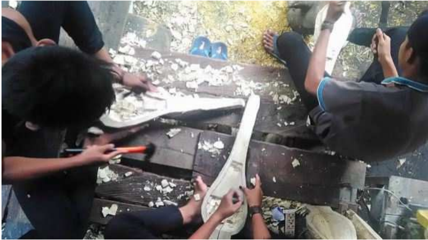
Hollowing the Panting soundbox by ALPI Wayang (Haruyan)
