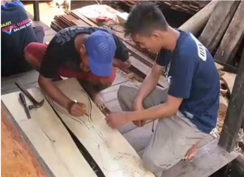
Unlike ALPIAN, the maker Fahrul ANWAR rather carves the cavity prior the outter shap.(Duba TV)
