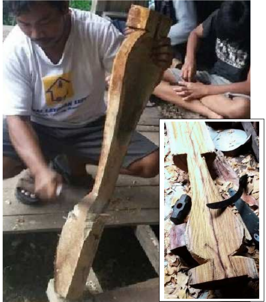
Outer carving of the wooden bodies (maker in Rantau)
