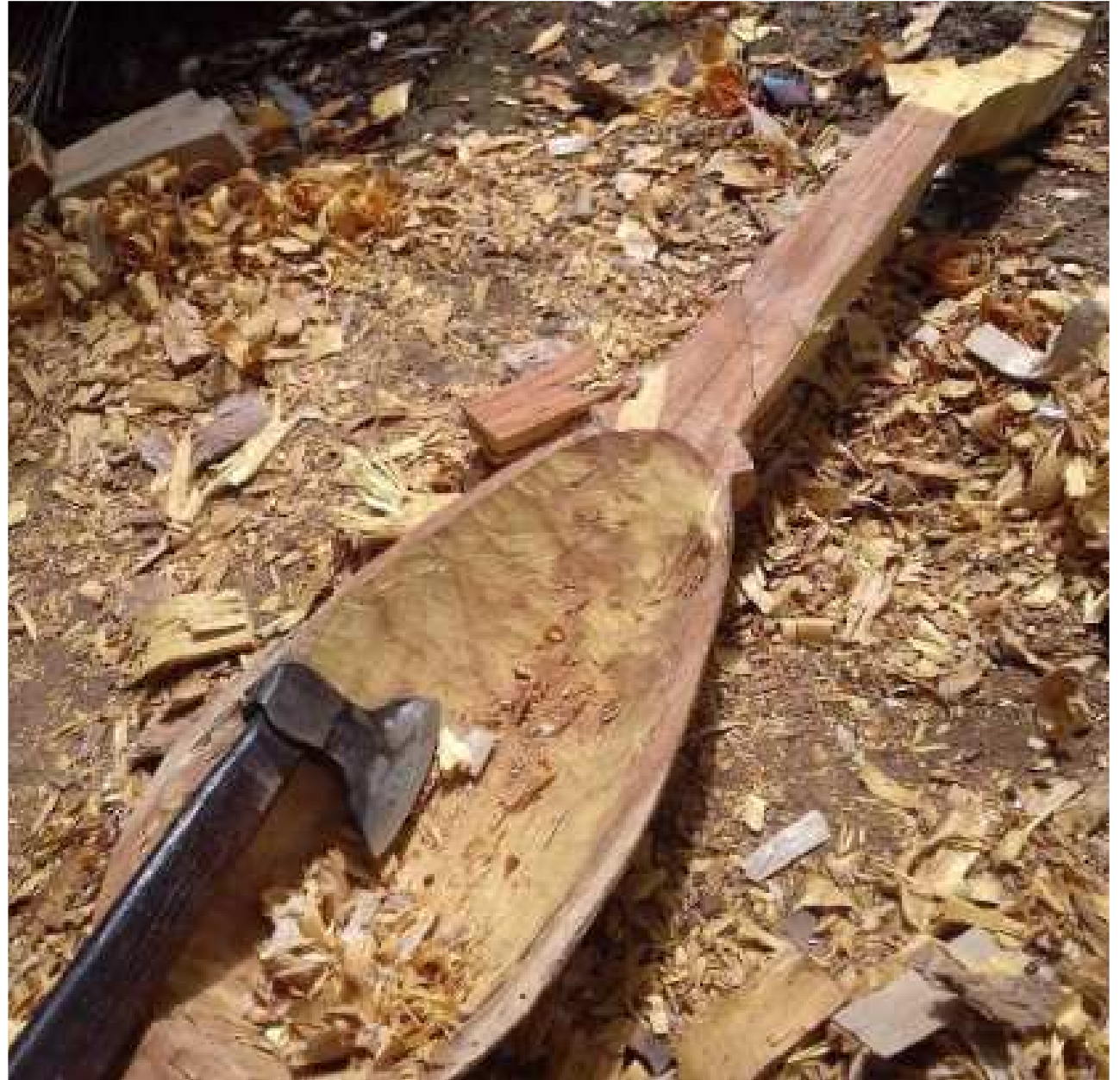
Shaping with the sabre, maker SYIR HAYATI
