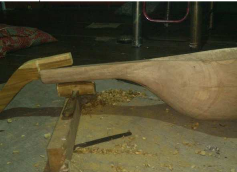
Panting pegbox assy: sizing the dovetail (maker RUDDY a.k.a. "RURUD", Barikin)
