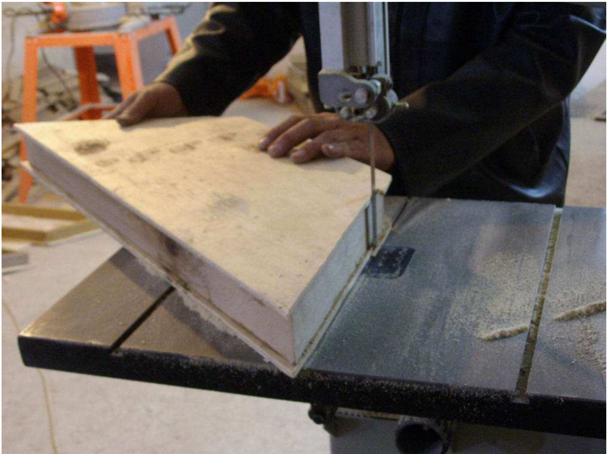
SHAPING THE SOUNDBOX : flattening the side-boards with an electrical saw
