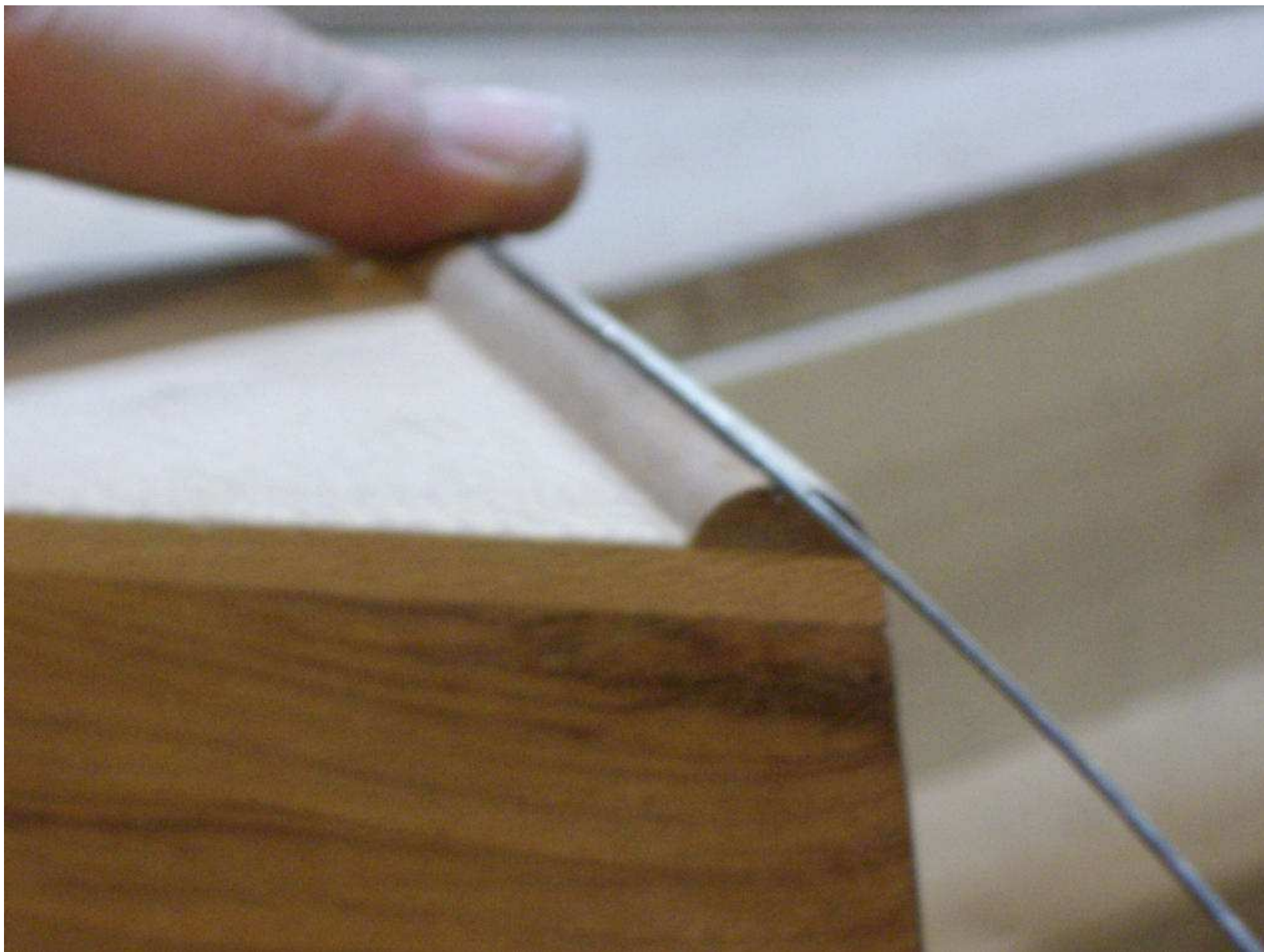
TIN FINISHER UPON THE « SHAYTANAK » : inserting a tin strip in the groove. According to VARZANDEH, the higher is the Shaytanak ( < 0,75'' ), the easier is the tuning, by moving Kharrak bridges.
