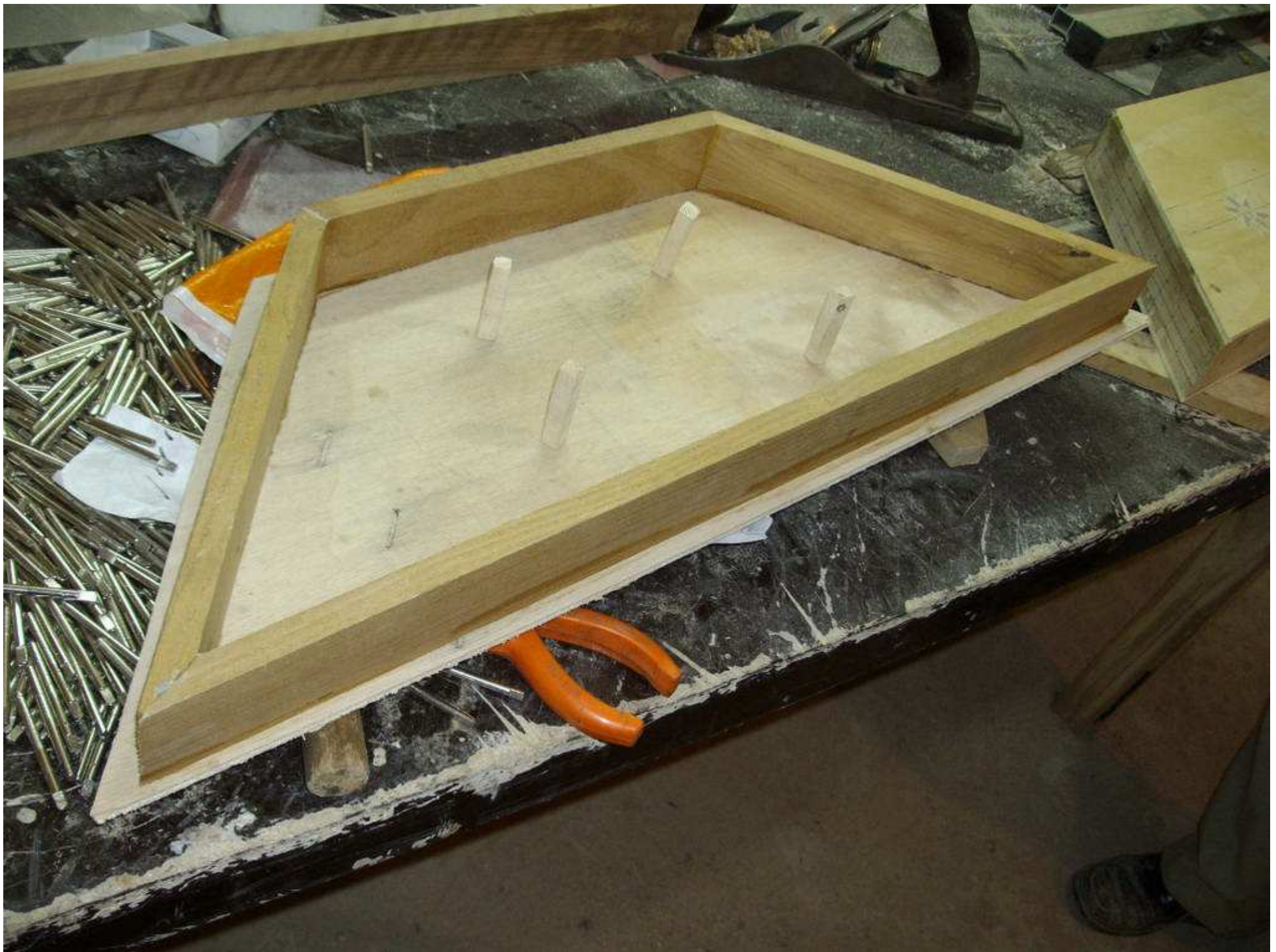
GLUEING PINEWOOD-MADE « POL » BRIDGES : variants exist , depending on wood quality ( 2, 3, 4 pols)
