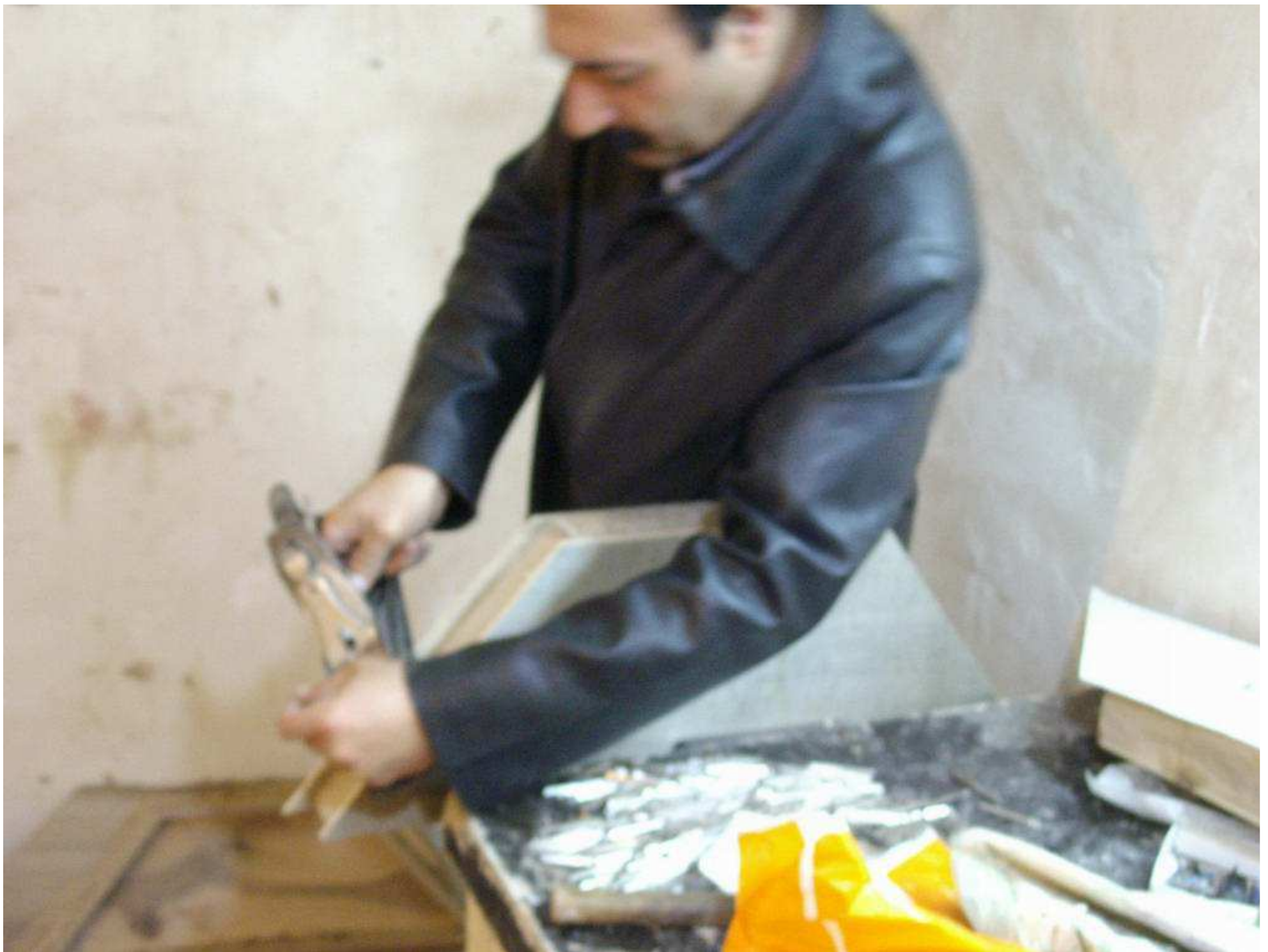
DEBURRING THE SOUNDBOX : flattening manually the side-boards
