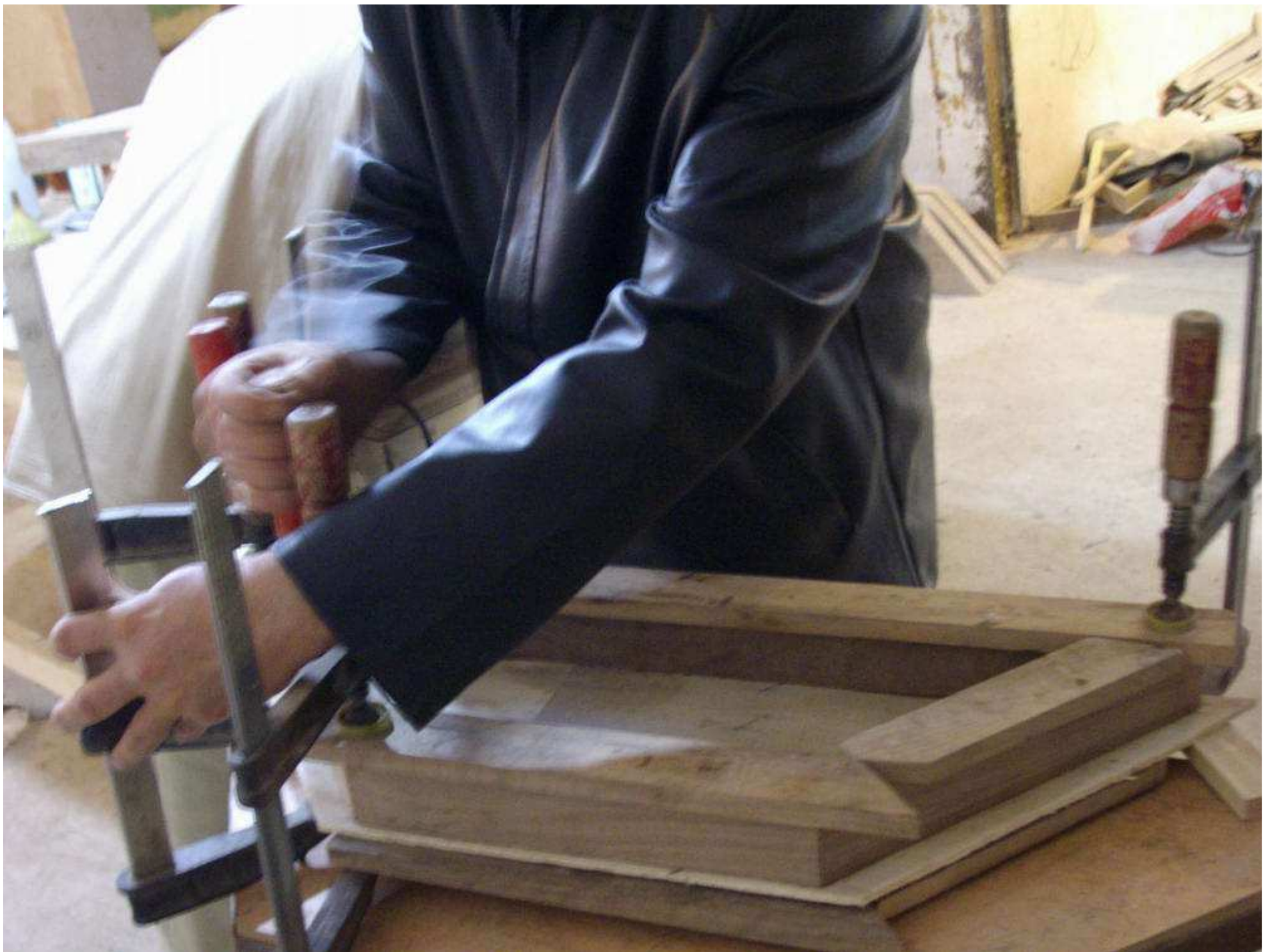
GLUEING THE SOUNDBOARD (4) : clamping the soundboard on frame, til them to be assembled.
