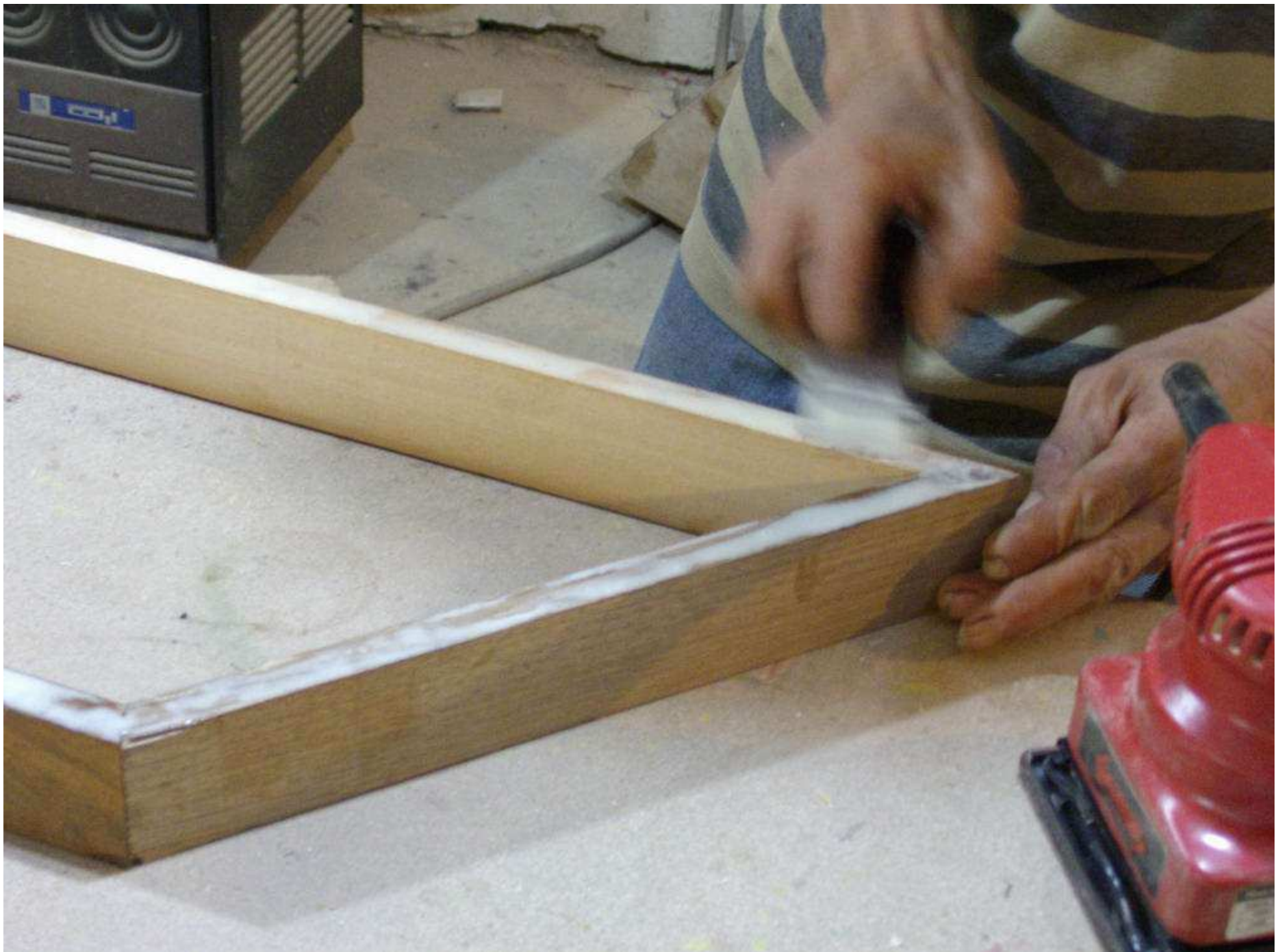
GLUEING THE SOUNDBOARD (1) : spreading the glue
