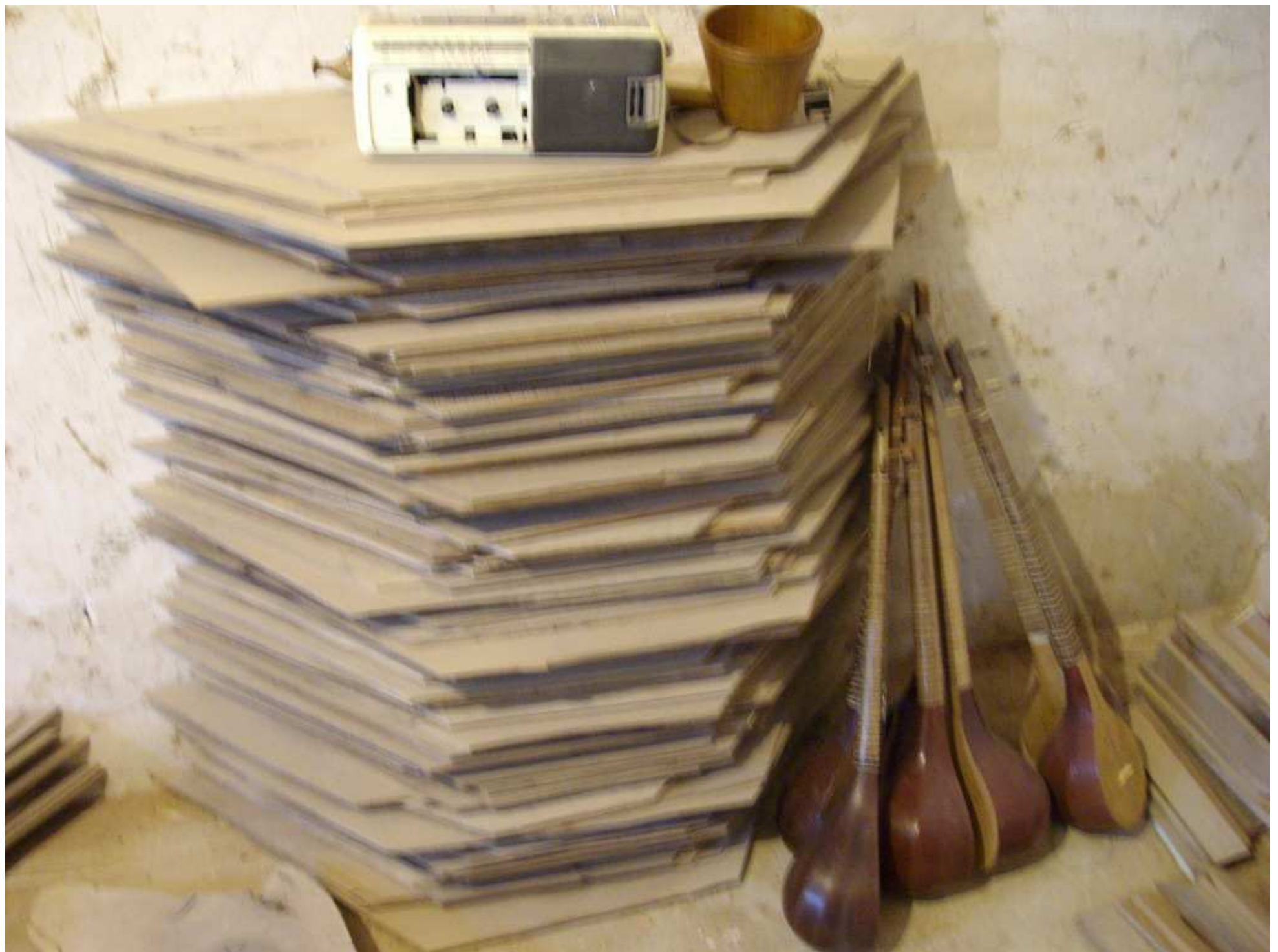
GLUEING THE SOUNDBOARD (3) : shaping 4mm thick boards out of geredu and tchub woodboards .
