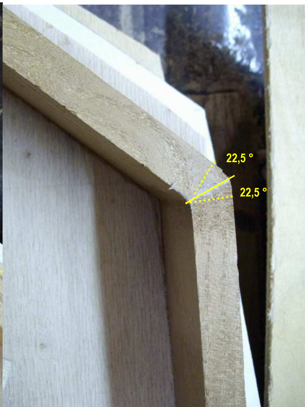
GLUEING WOODEN FRAME : preadjustment is frozen thanks to a pneumatic staple-fitter. Item illustrated here is made of high quality geredu wood
