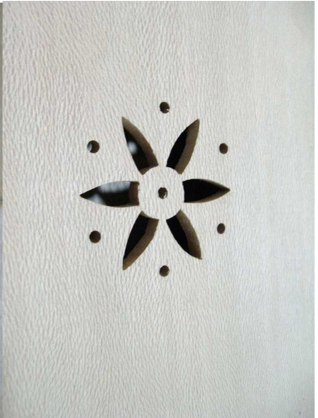
CARVING SOUNDBOARD OUTLETS (3) : in progress with gouge ; right : a geredu wood made soundboard.
