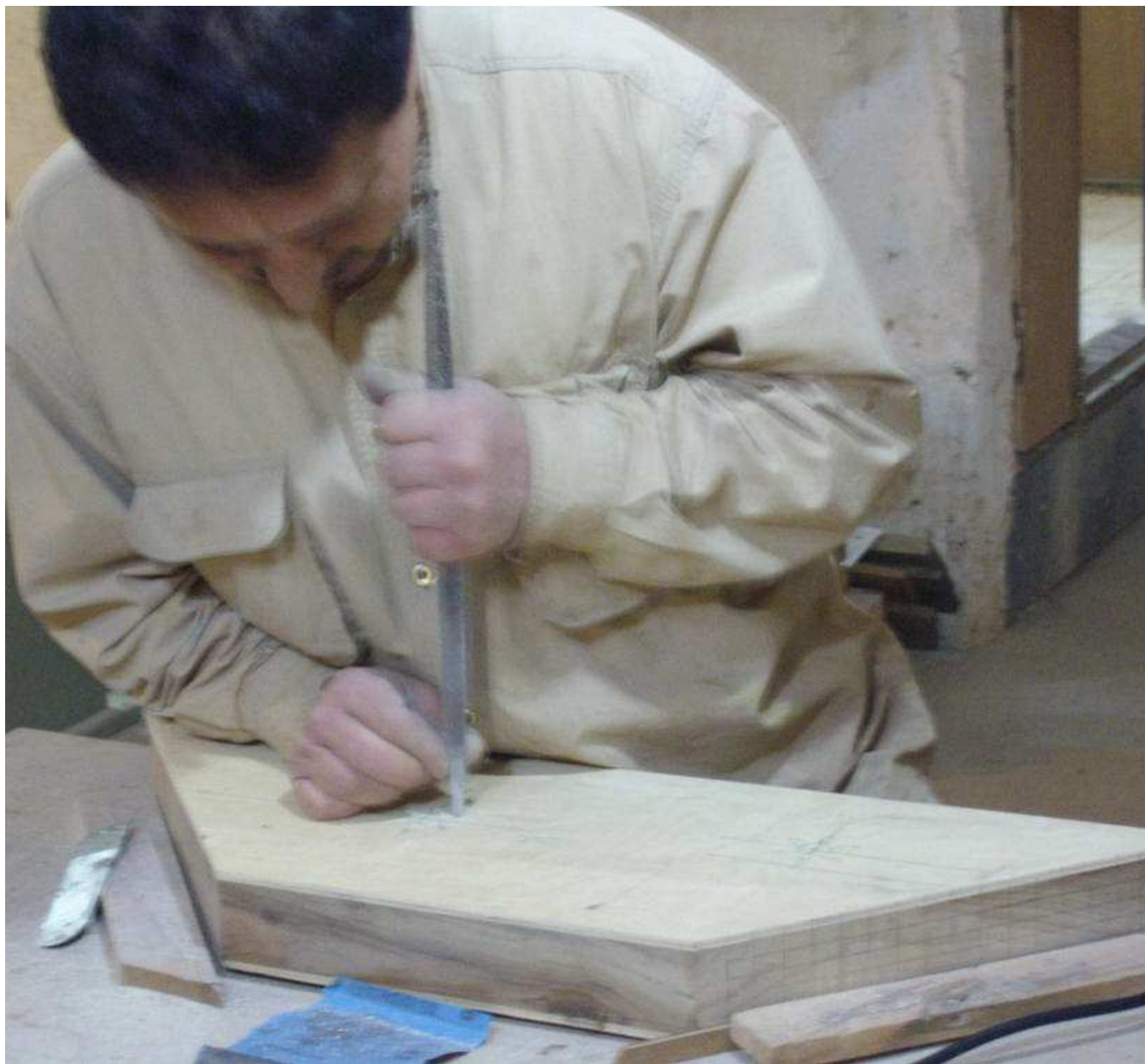
CARVING SOUNDBOARD OUTLETS (2) : with gouge.
