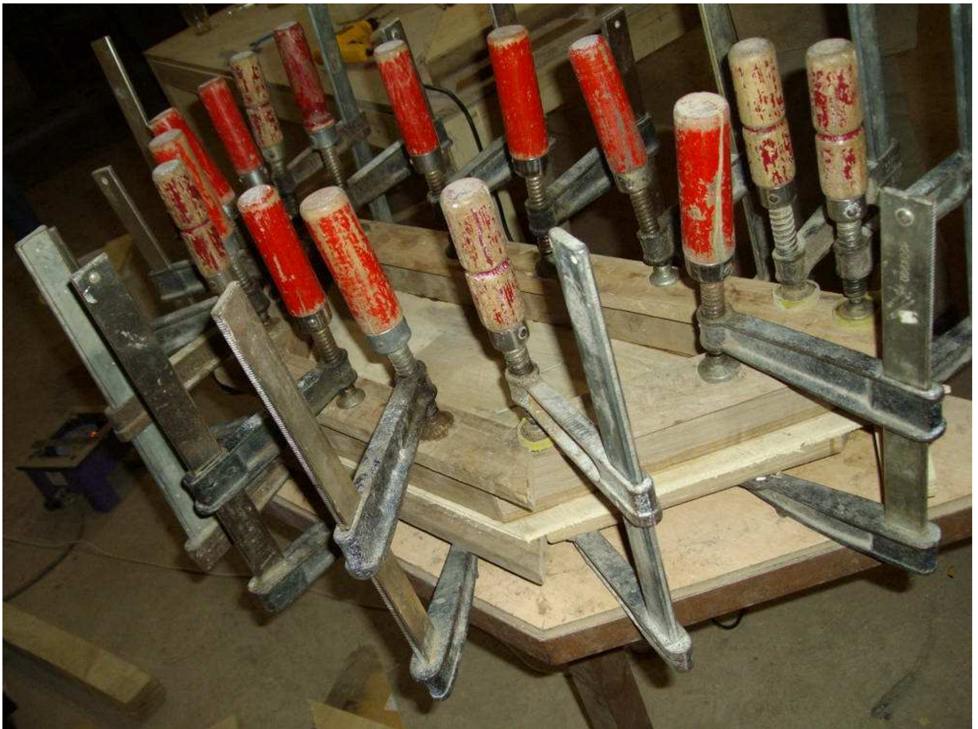
GLUEING THE 2 ND SOUNDBOARD : on a clamping table. Recommended thickness for base board is 6 mm.
