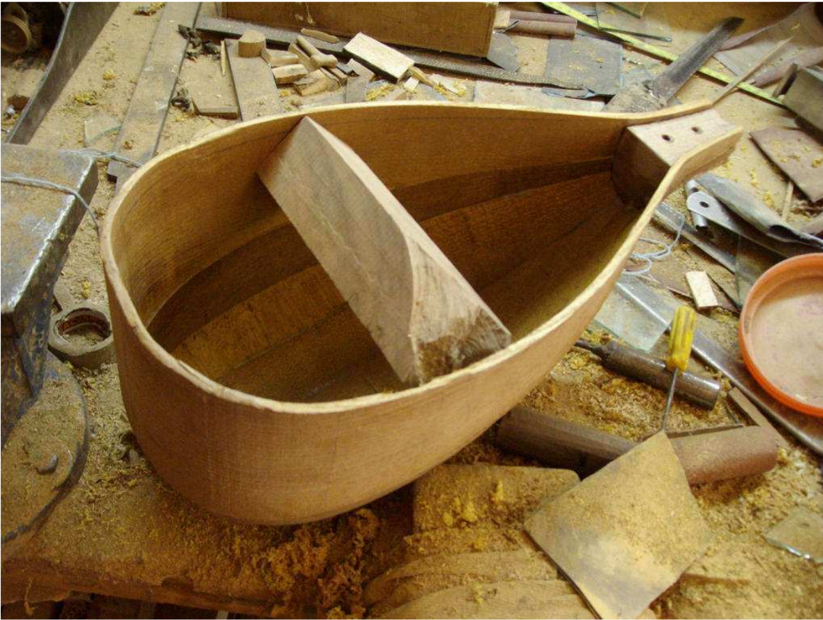
Rib-made tanbur soundbox. The usual technics for setar was extended to cheap Tanbur constructions. Maker Fereydun KAMALI , Kerend, Dalahu.
