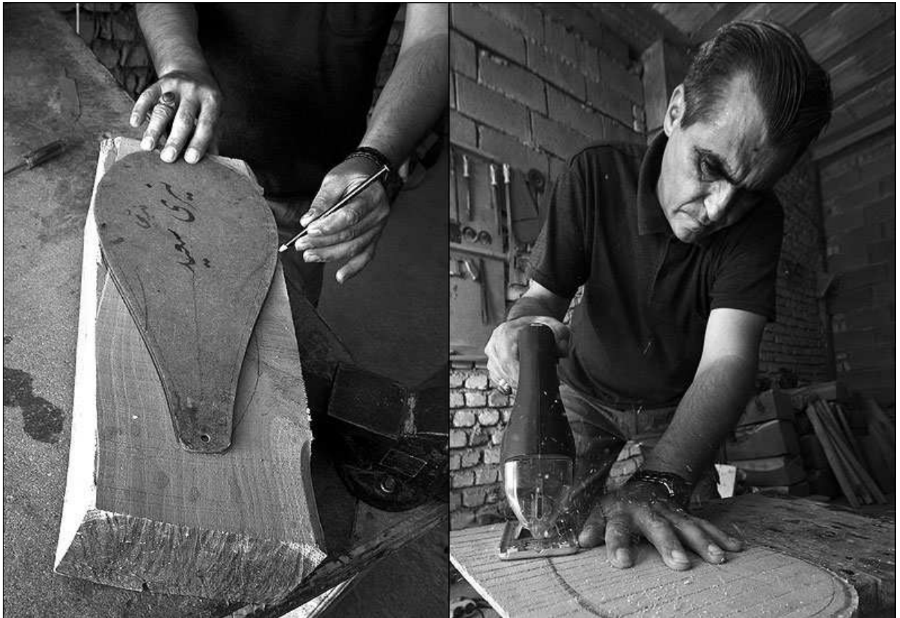
The soundboard is shaped out of flexible wood sheet ( source web x).
