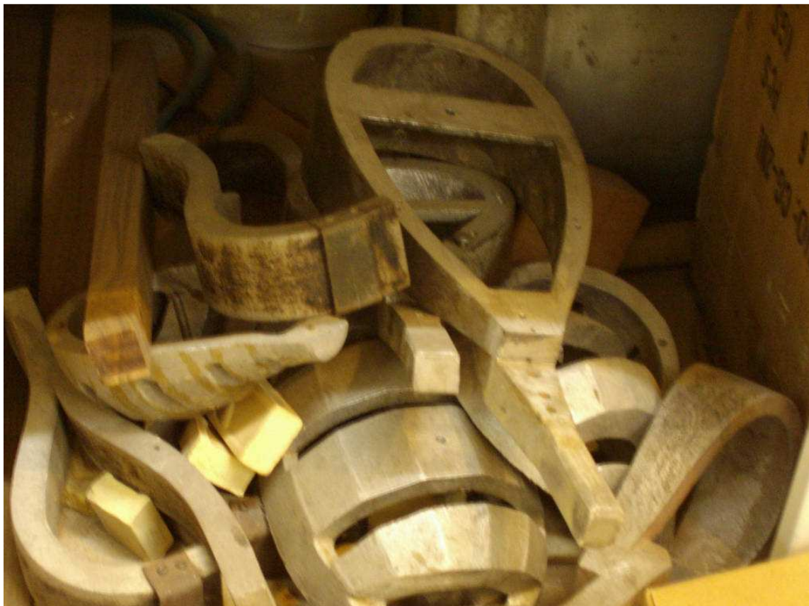
Tanbur application: shaping pattern and clamp for Tanbur ribbed soundbox. Maker POURAM , Kermanshah.
