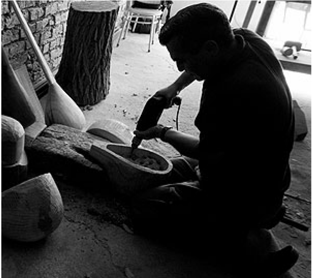
Carving the soundbox by combination of the gouge and driller ( source web x).
