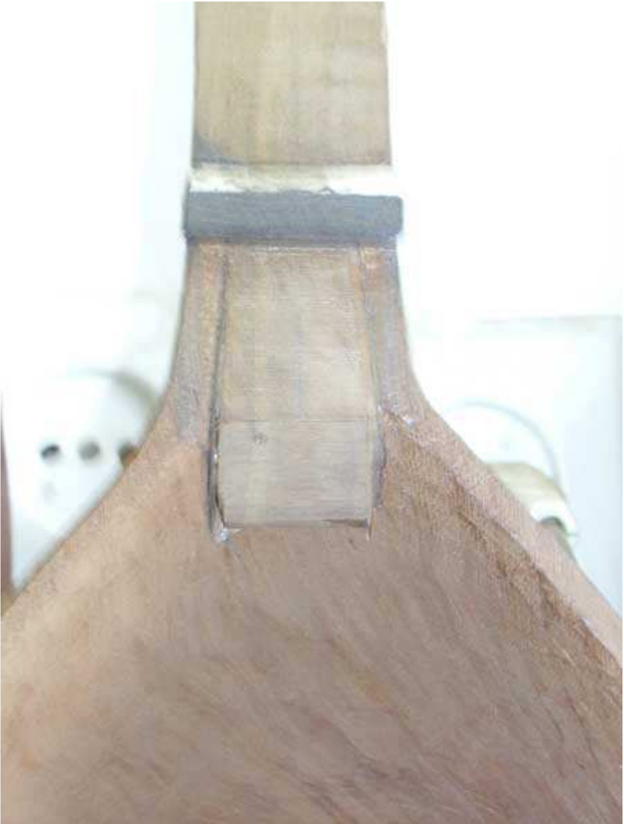
Joining Sounbox & Neck ( glue) : As observed at Ali Reza RAHNIM s , Qasvin. Considering the absence of strengthener, the junction structure is much more simple than the design by POURSHAGHAGHI for rib-made box ( see INSERT 0082).
