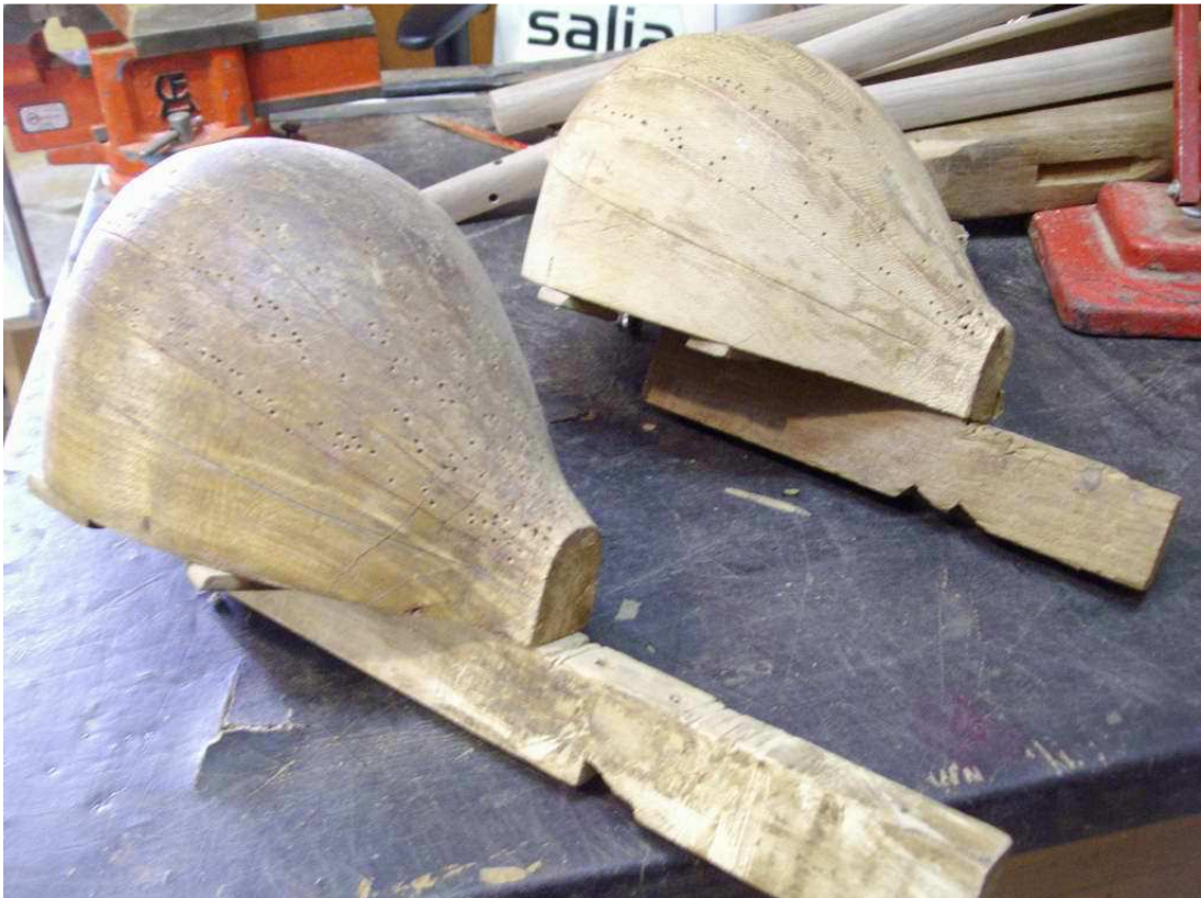
Bending patterns for Setar ribbed soundbox. These items allow adjusting the neck alignment too. Cultural Heritage Organization Center, Tehran
