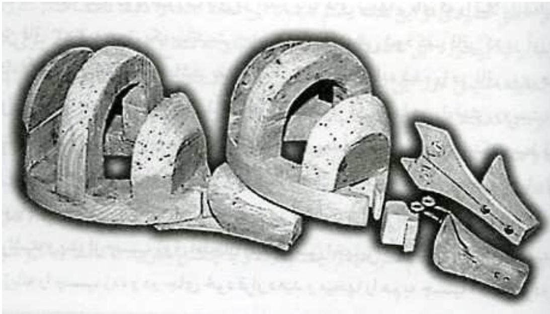
Bridged Mold by H. MASOUD . The tongue section is screwed on a removable plate.
