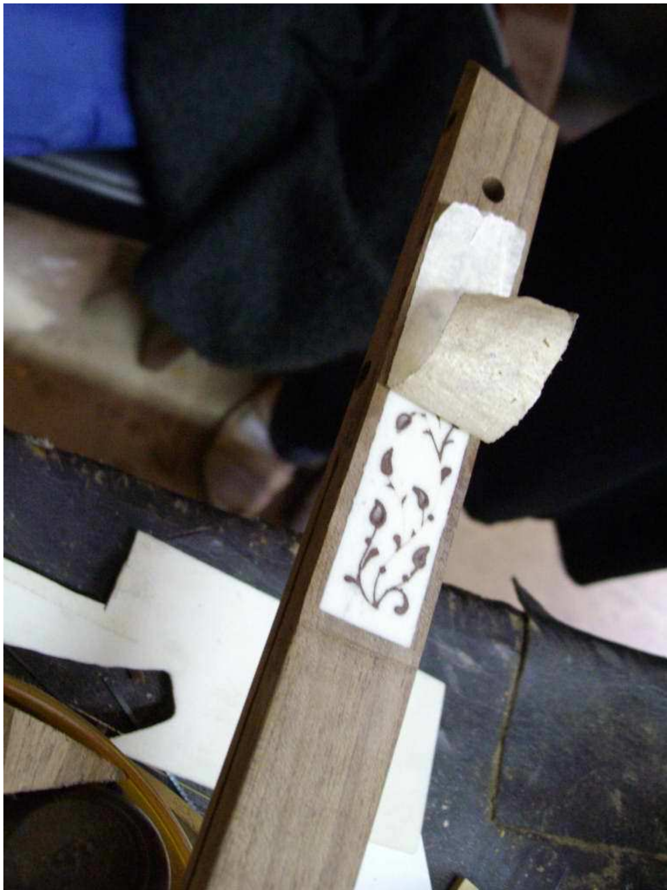
Ornamentations are carved in ivory with a micro-saw. Then the ivory plate is adjusted in the cavity. (Cultural Heritage Organization Center, Tehran )
