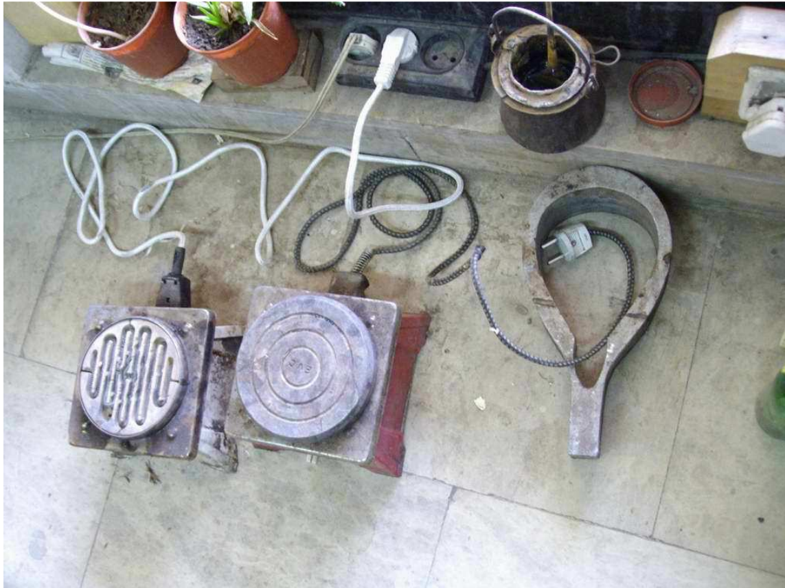
Bending pattern & heaters for Setar ribbed soundbox. Cultural Heritage Organization Center, Tehran
