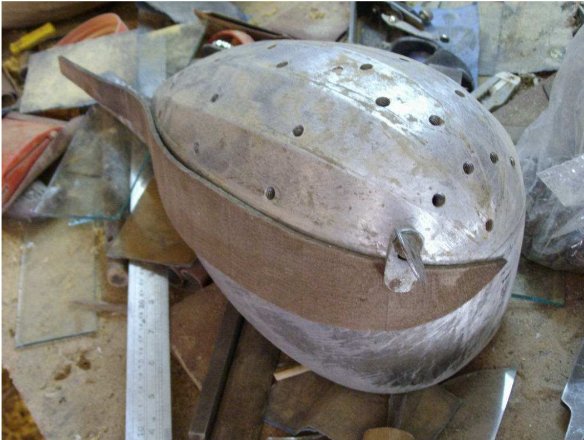
Tanbur application: shaping pattern & clamp for Tanbur ribbed soundbox. Maker Fereydun KAMALI , Kerend, Dalahu
